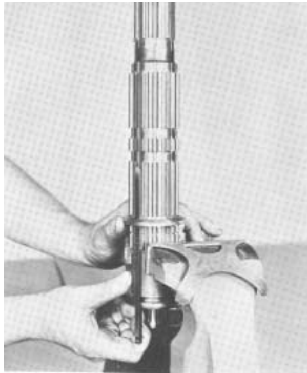
#86 - Installing reverse gear washer on shaft and inserting key through keyway and washer.
