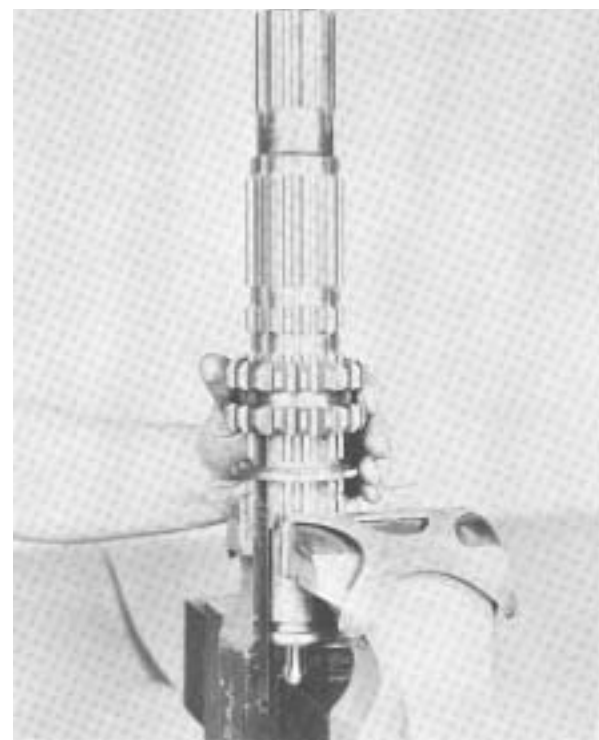
#87 - Installing the 1st-Reverse sliding clutch gear on shaft.
