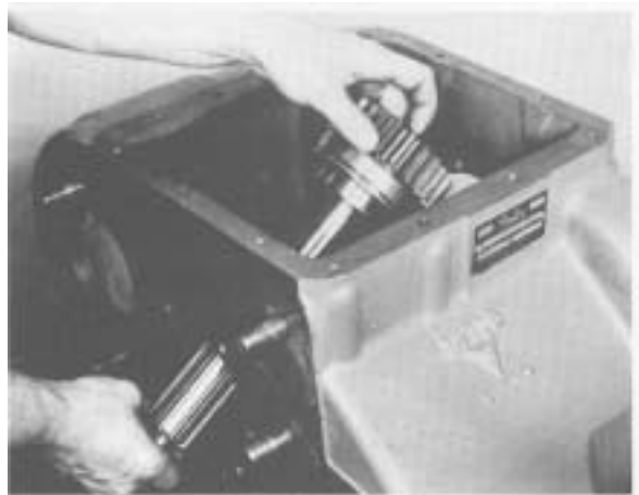
#51 - Lifting gear assembly out through top of case.
