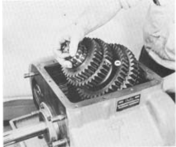
#107 - Lowering mainshaft in position in case; mesh corresponding gears on left countershaft with those on mainshaft.
