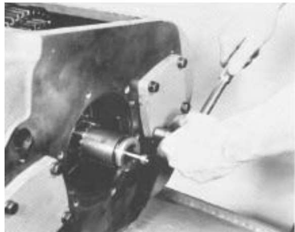
#24 - Removing rear bearing cover from right countershaft.
