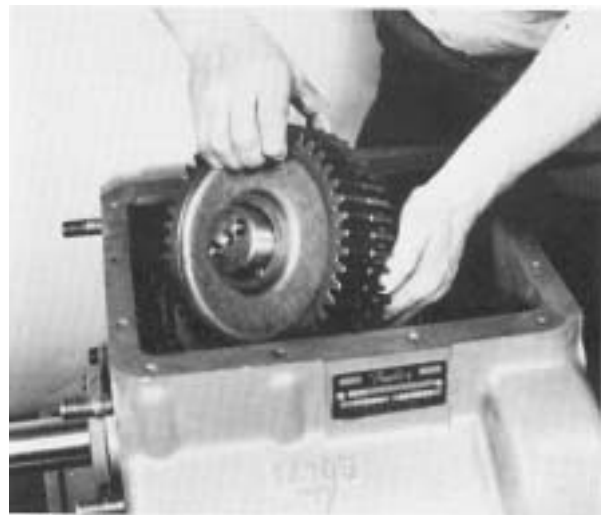
#82 - Placing the right countershaft into position in case. Do not install bearings.
