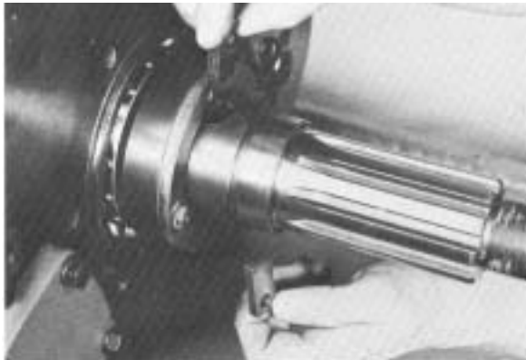
#129 - Installing flat keys in tailshaft to engage slot in mainshaft.
