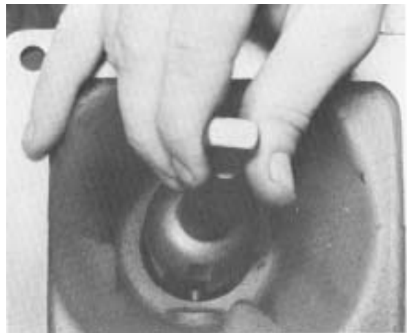
#149 - Installing the gear shift lever in housing.
