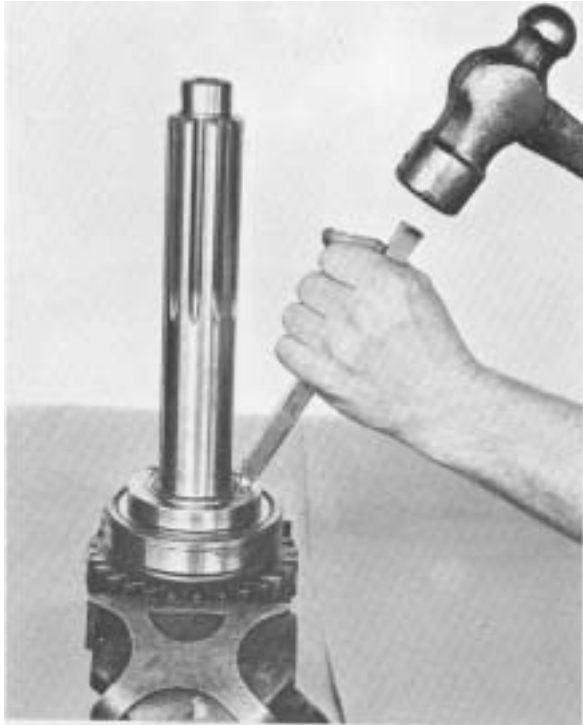
#52 - Relieving bearing nut where peened into shaft.
