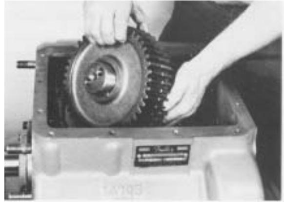
#39 - Lifting the right countershaft from case.
