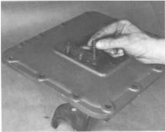
#145 - Installing the three tension springs in bores.
