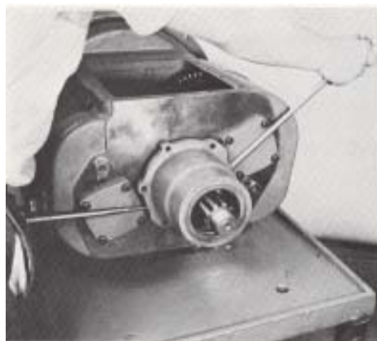
#10 - Prying rear bearing cover evenly to rear.
