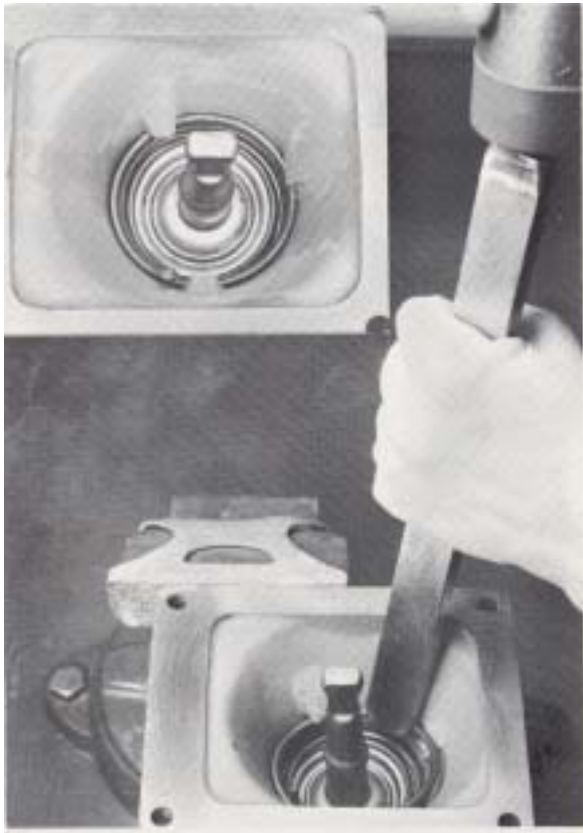
#151 - Installing tension spring in housing, fitting spring under lugs cast inside the housing.
