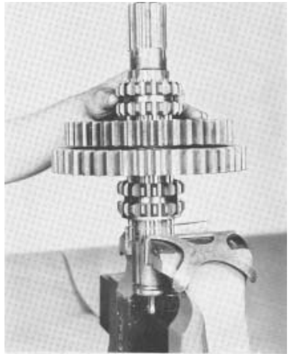
#94 - Installing the 2nd-3rd speed sliding clutch on shaft.
