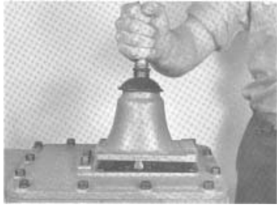
#1 - Lifting gear shift lever housing from shifting bar housing.
