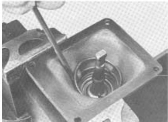
#2 - Removing the gear shift lever tension spring from under lugs cast in housing.
