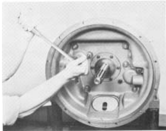
#18 - Turning attaching bolts from clutch housing.
