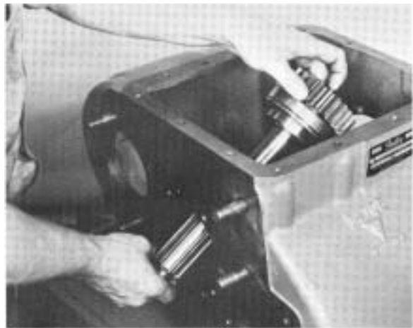
#63 - Installing the drive gear assembly through top of case.
