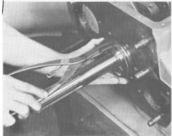
#50 - Removing snap ring from drive gear bearing.
