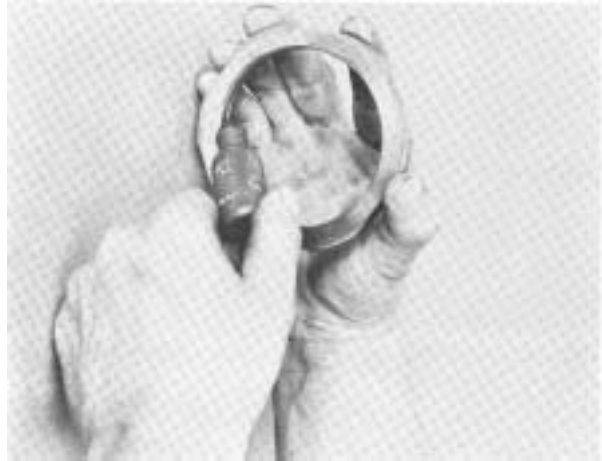
#124 - Applying Loctite to threads of bearing nut.
