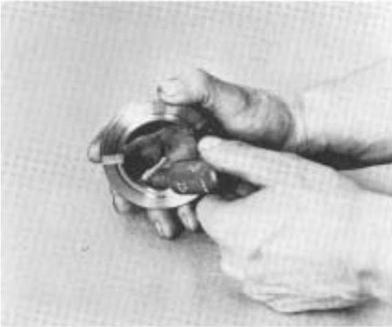
#59 - Applying Loctite sealant to threads of drive gear nut.
