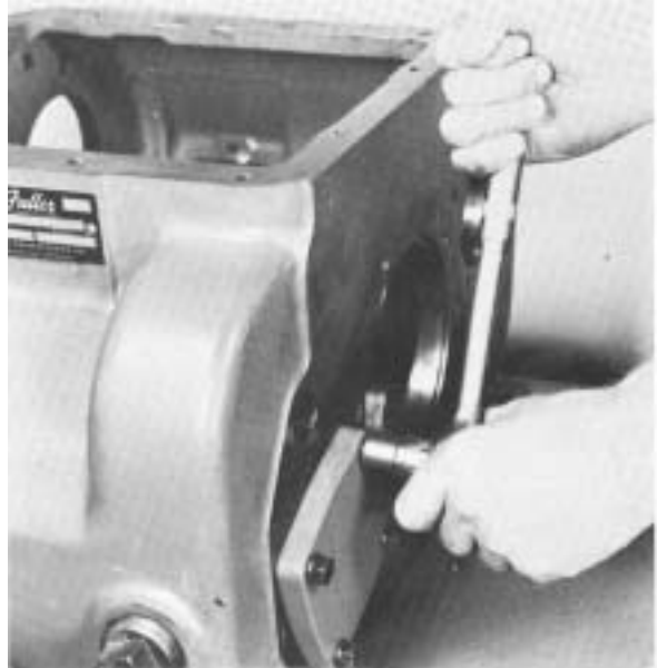
#42 - Removing rear bearing cover from left countershaft.
