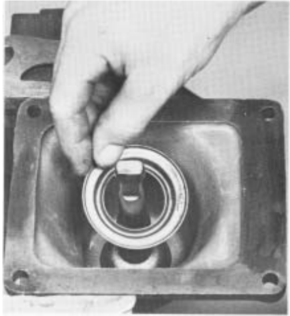
#150 - Installing the tension spring washer in housing.
