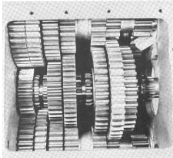
#108 - Mainshaft assembly in correct position in case.
