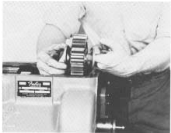
#23 - Removing left reverse idler gear and the two thrust washers from case.
