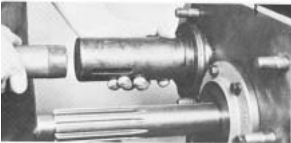
#111 Installing front bearing on right countershaft.
