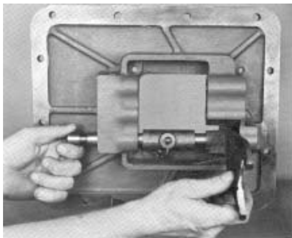
#138 - Installing the 1st-Reverse speed shift bar and shifting yoke and block.
