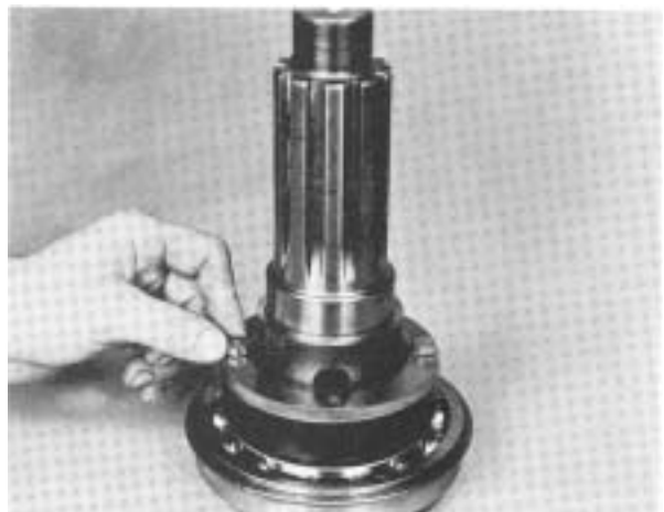
#126 - Installing key-spacer ring on tailshaft.
