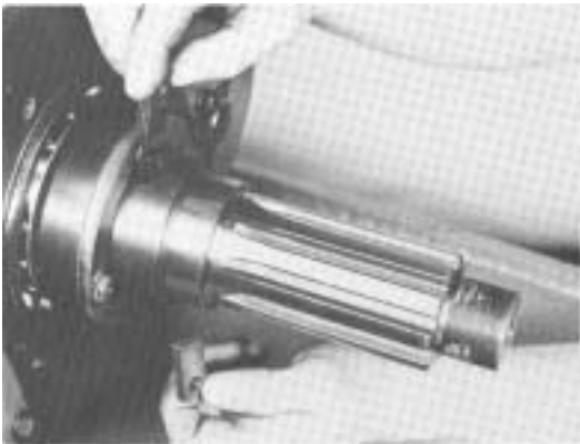
#14 - Removing flat keys from tailshaft. These keys maintain relative position of mainshaft to tailshaft.
