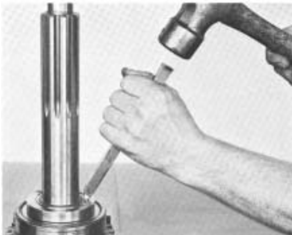
#61 - Peening nut into the two milled slots of shaft.
