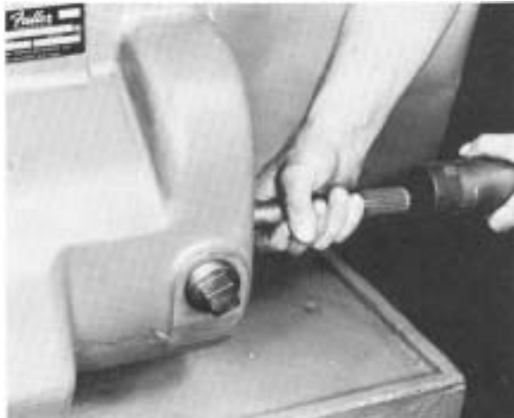
#45 - Moving left countershaft forward to unseat from bearing.
