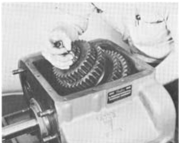
#30 - Removing mainshaft assembly from case.
