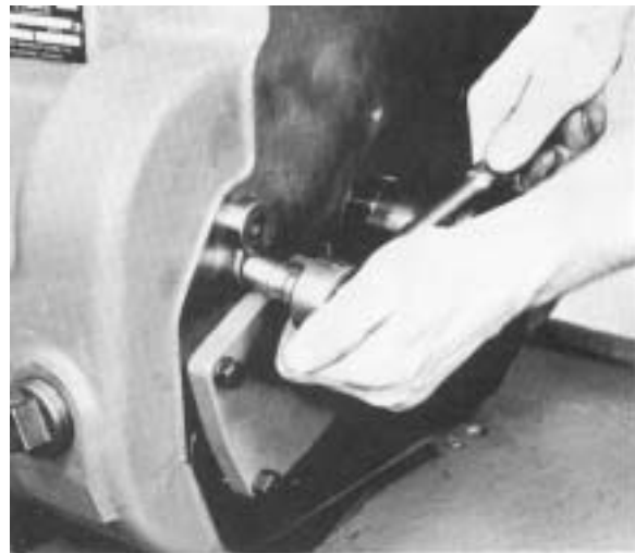
#117 - Installing lockplate in reverse idler shaft.
