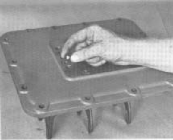
#144 - Installing tension balls in bores on top of housing.
