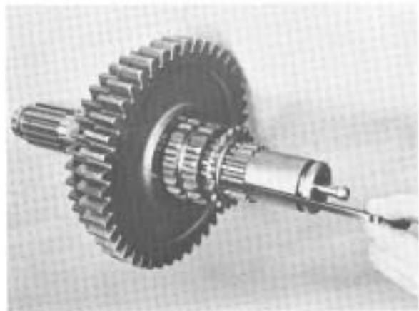
#35 - Pulling the long key from mainshaft.
