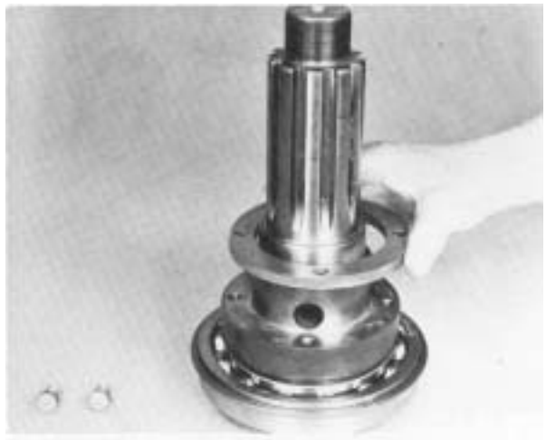
#16 - Removing key spacer ring from tailshaft.
