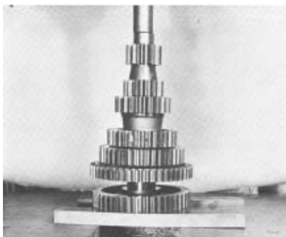
#71 - Pressing the drive gear on countershaft.
