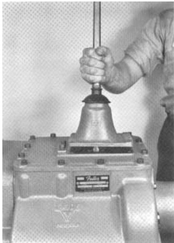
#152 - Installing the gear shift lever housing on shifting bar housing.
