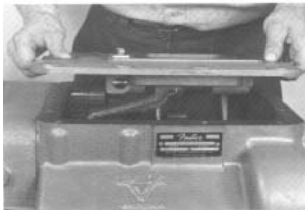
#4 - Lifting the shifting bar housing from transmission.
