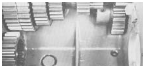
#106 - The right countershaft moved towards case wall.
