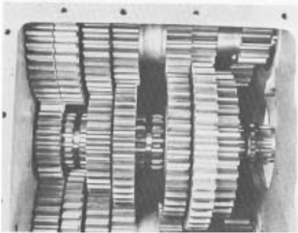
#109 right countershaft moved into position to mesh with gears of mainshaft. Timing tooth on drive gear must mesh with timing teeth on main drive gear.
