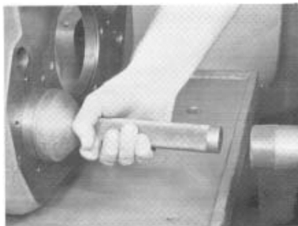
#76 - Installing rear bearing on left countershaft.
