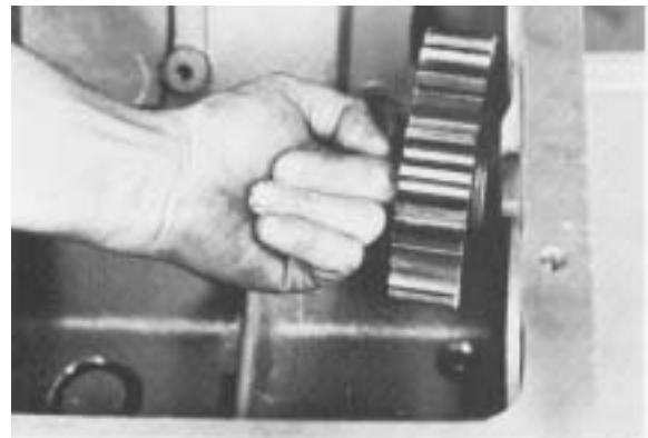
#41 - Removing the right reverse idler gear and two thrust washers from case.
