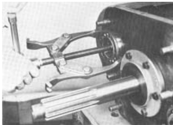
#29 - Pulling from bearing from right countershaft.
