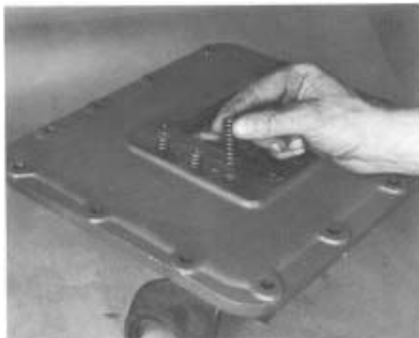
#5 - Removing shifting bar tension springs.
