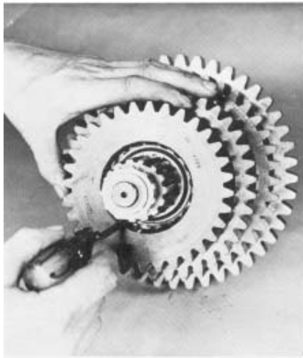
#100 - Installing the 4th speed gear washer on shaft and aligning keyway in washer with keyway in shaft.
