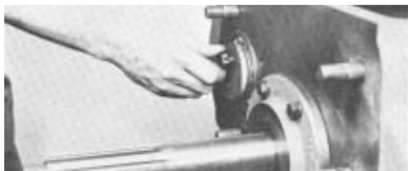
#112 Installing bearing retainer plate on front of right countershaft.
