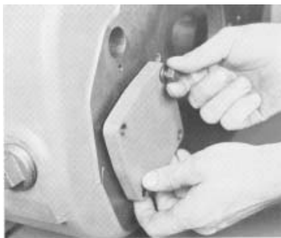
#79 - Installing rear bearing cover.
