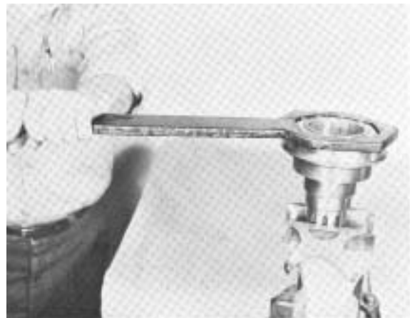
#17 - Turning bearing nut from tailshaft, left-hand thread.
