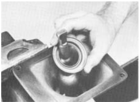
#3 - Removing washer and gear shift lever from housing.
