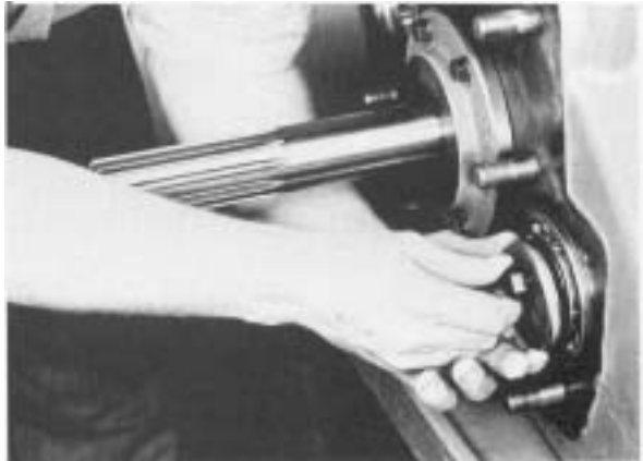
#43 - Removing bearing retainer plate from front of left countershaft.
