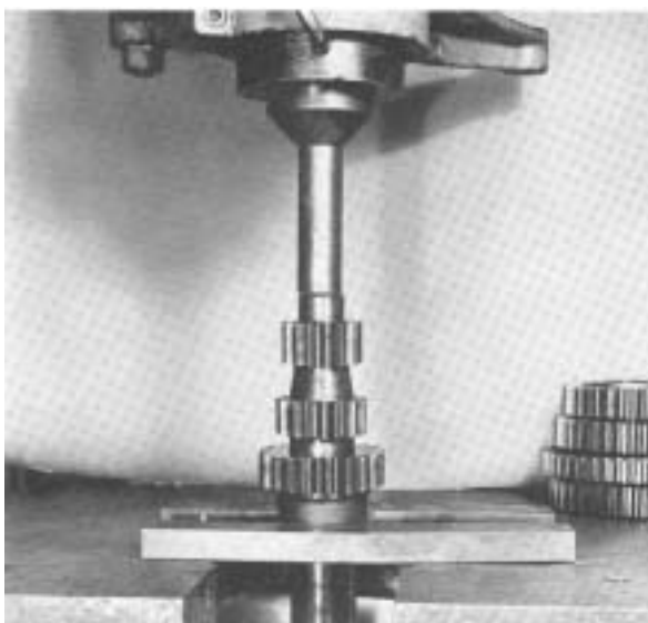
#68 - Pressing the 2nd speed gear on countershaft.
