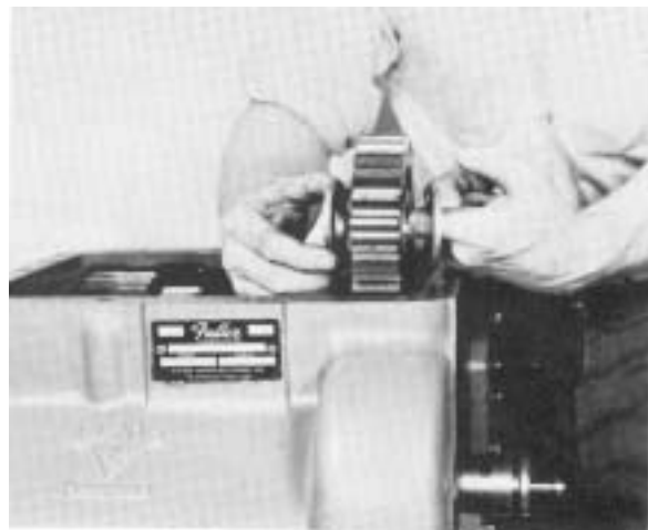
#115 Place the two thrust washers and reverse idler gear into position in case.
