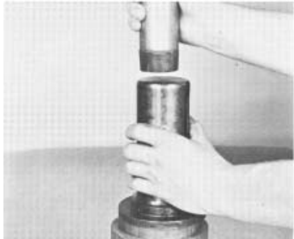
#134 - Installing oil seal in rear bearing cover.
