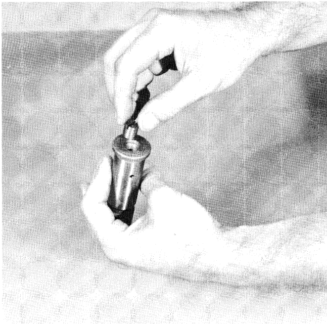
1. Install the plug in the end of the reverse idler shaft.
