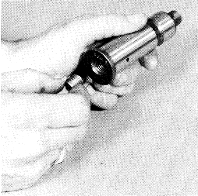
1. Install the plug in the idler shaft.
