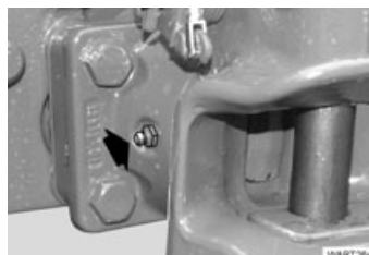
Automatic trailer hitch with cylinder-type bolt.
