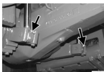
Bottom lift cylinder bearing of front axle suspension.
