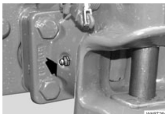
Automatic trailer hitch with cylinder-type bolt.
