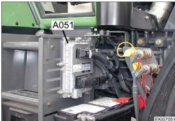
Measuring point on A051 - ECU, engine control unit (X1466 - separation point)
