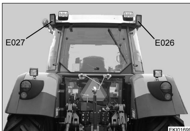
E026 = Indicator high-mounted right rear E027 = Indicator high-mounted left rear Tractor seen from rear
