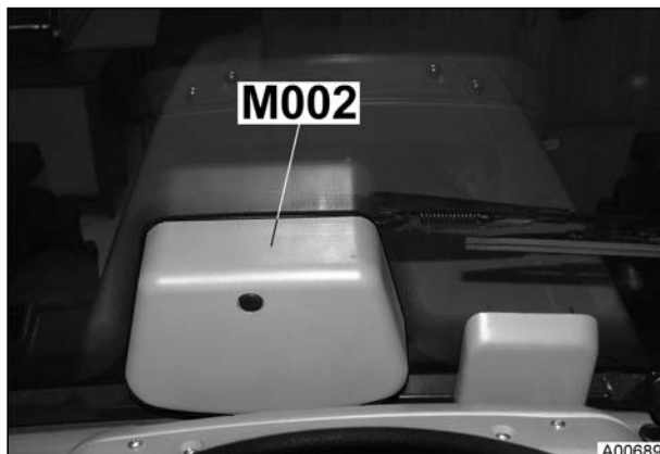
M002 = Wiper motor, front In windscreen
