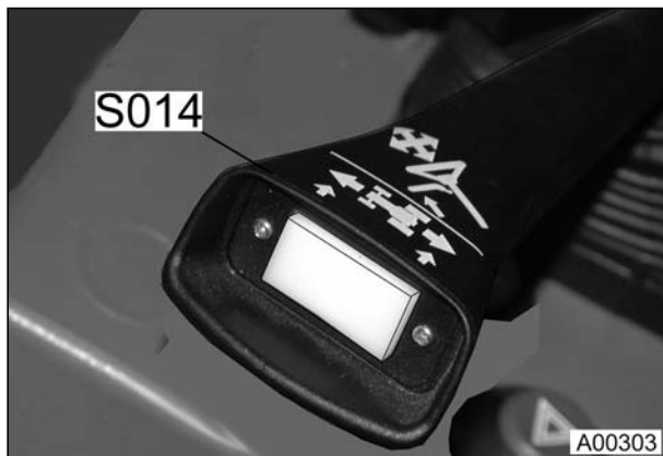
S014 = Switch, rapid reversing To left of steering wheel
