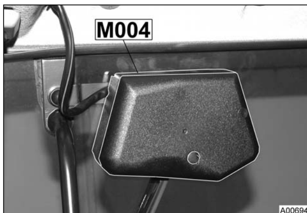
M004 = Wiper motor, rear In rear window
