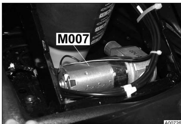
M007 = Motor, seat adjustment Under seat bracket
