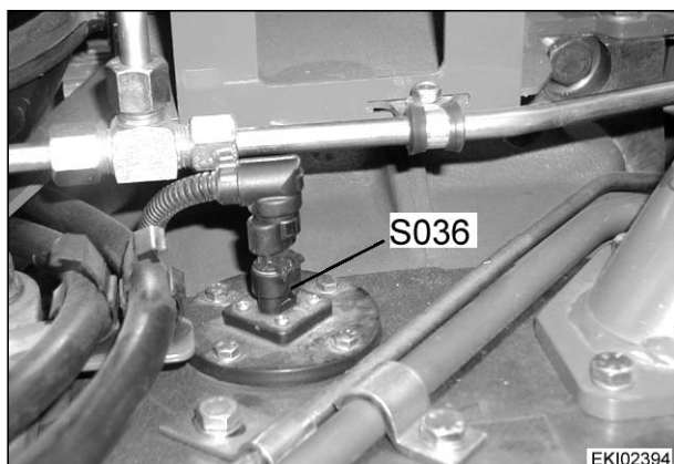
S036 = Switch, hydraulic oil level On top of clutch housing
