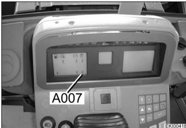
A007 = Display unit At top of steering column
