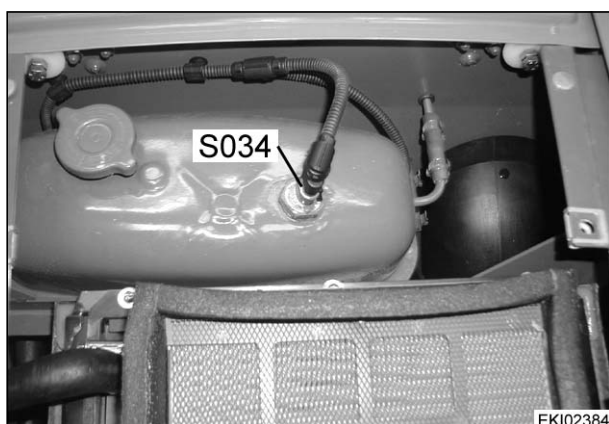
S034 = Switch, coolant level Expansion tank at rear of engine compartment
