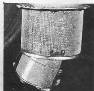
Removing oil filter and screen.
