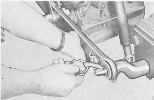
Fig. 26 - Attaching Left Lower Link to Implement
