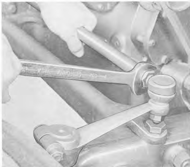
Fig. 80 - Adjusting Drag Links
