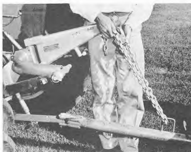
Fig. 30 - Installing Coupler Chain to Implement
