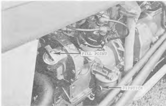
Fig. 13 - Crankcase Oil - Check and Fill Points
