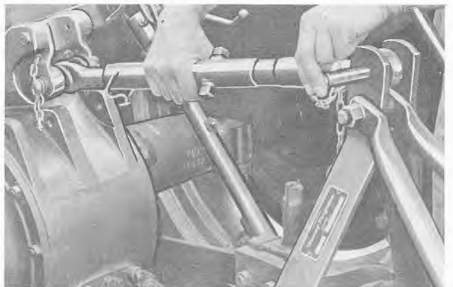
Fig. 28 - Attaching Top Link
