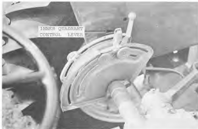
Fig. 23 - Using Position Control
