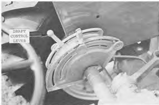
Fig. 21 - Using Draft Control
