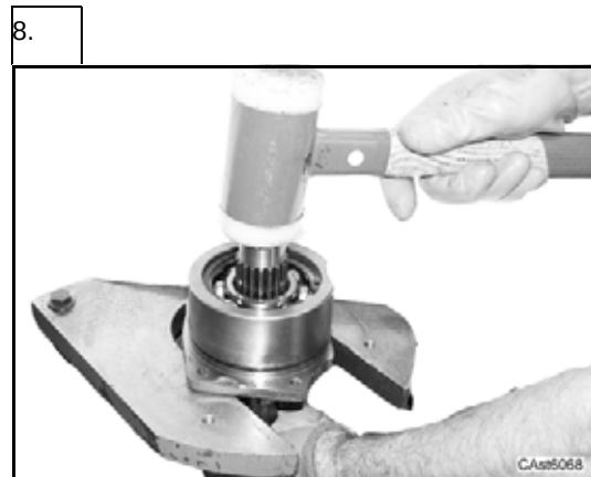
Pull out shaft (6) by means of an hammer.
