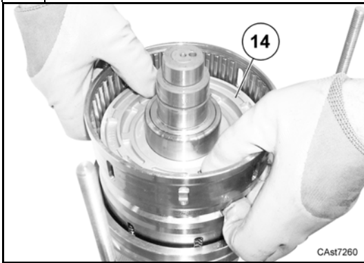
Assemble piston (14) in its seat.
