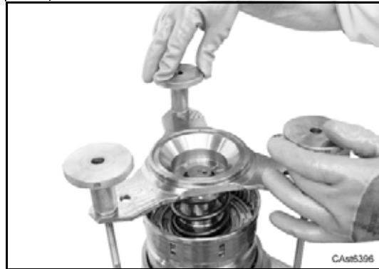
Assemble bush "CA715791" on page 324 and upper cover of tool "CA715358" on page 324.
