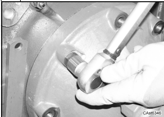
Tighten fastening screws of final drive to the requested torque.
