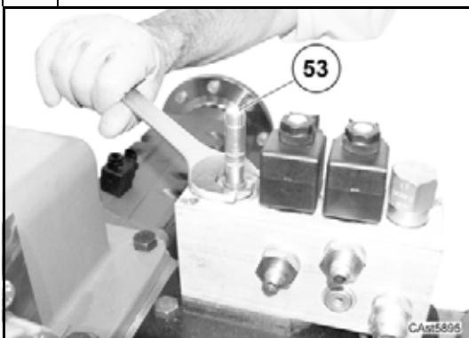
Assemble valves (53) with relevant O-Rings.
