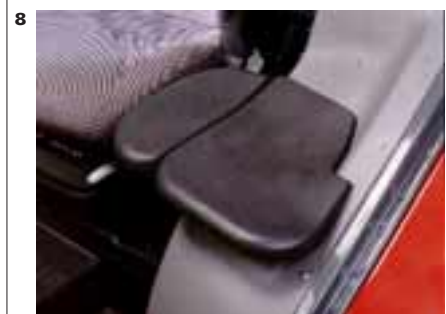
Fig. 9. 'Versa' cab with 180° swivel seat and rear operator's footwell
