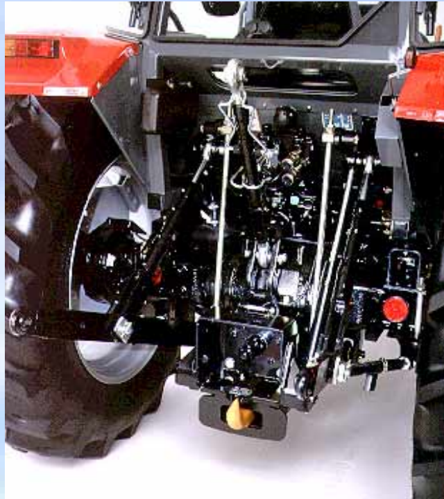
Left: Adjustable screw stabilisers as standard give better control and easier adjustment of implement lateral movement
