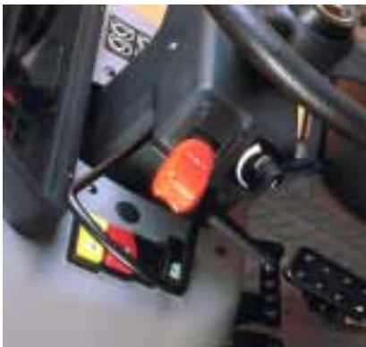
Left: The PowerShuttle lever is guarded to avoid accidental engagement. The Comfort Control switch is conveniently located
