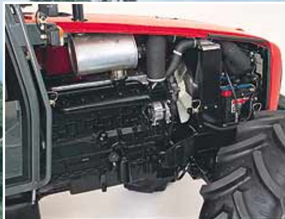
Below: The MF 4270 fitted with the Perkins 1000 Series 6-cylinder engine, shown left, offers outstanding performance
