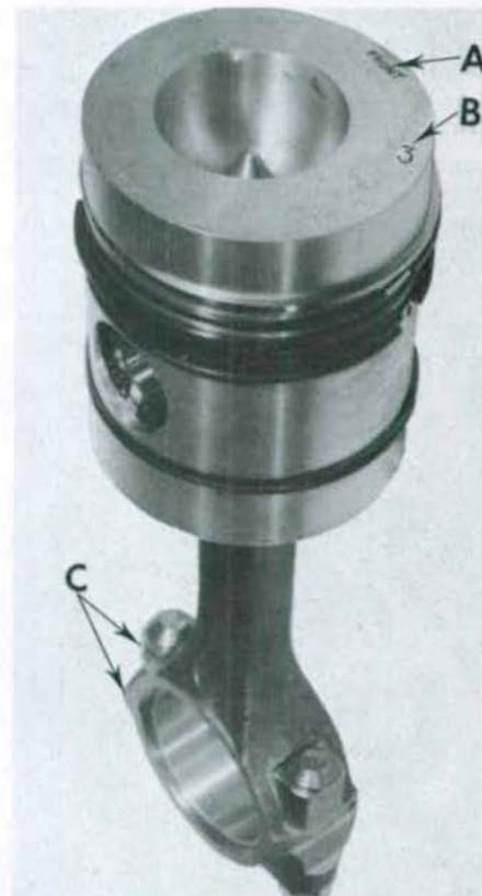
Fig. 71—Assemble rod and piston units as shown.
