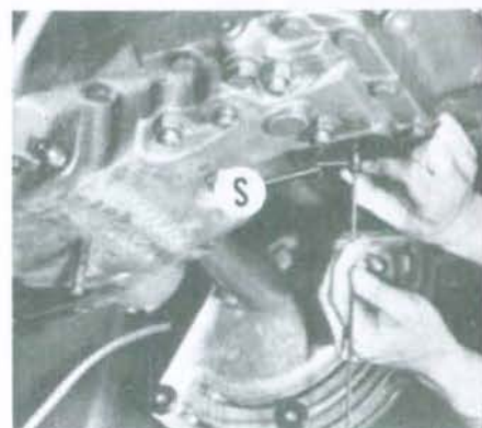
Fig. 208—Standpipe (S) can be guided into position with a piece of welding rod as shown.
