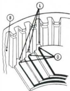
Fig. 152—Cross-sectional view of Multi-Power clutch showing recommended method of assembly. Refer to text.
