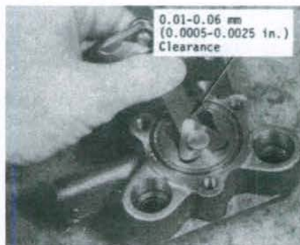
Fig. 79—Clearance between inner and outer rotors can be measured using a feeler gage as shown.
