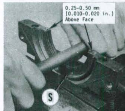
Fig. 77—Use a round bar to seat the rope seal into retainer half. The slot (S) is only in lower half of seal retainer. Do not trim ends of seal.
