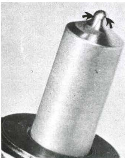
Fig. 88—Nozzle holes (arrows) are not located at an equal distance from nozzle tip.
