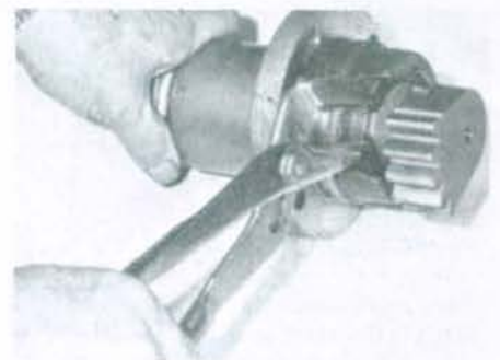
Fig. 7—The snap ring must be removed as shown before pitman shaft can be removed from housing.
