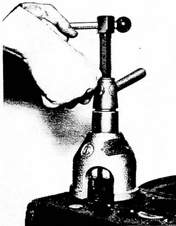
FIG. 116 REMOVING VALVE SEAT INSERT SERVICE TOOL MF540
