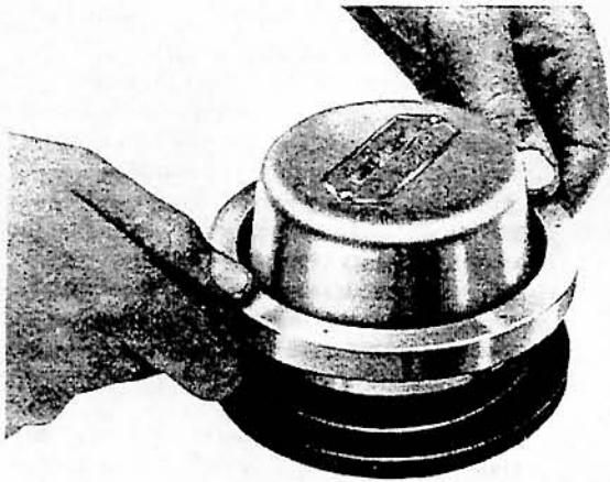
FIG. 146 FITTING NEW REAR OIL SEAL ON TO ADAPTOR MF105C/2 USING MF105C/1 AS GUIDE
