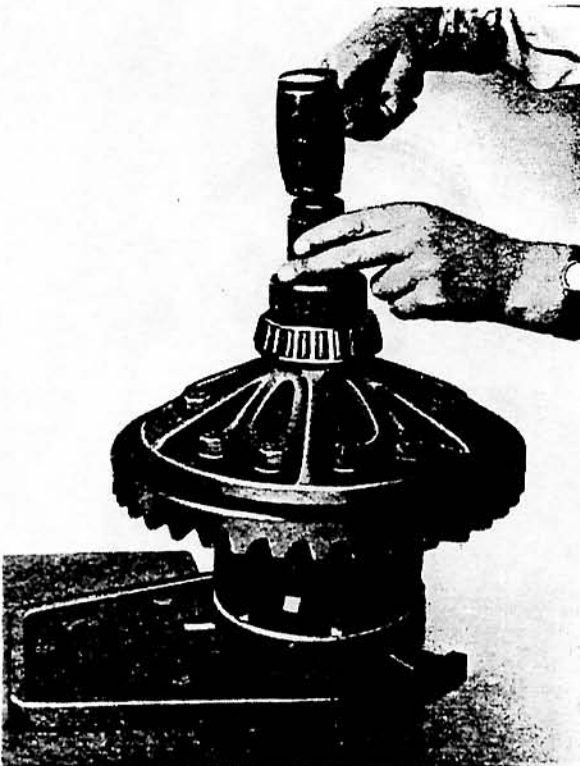
FIG. 15 REPLACING DIFFERENTIAL BEARING CONES
