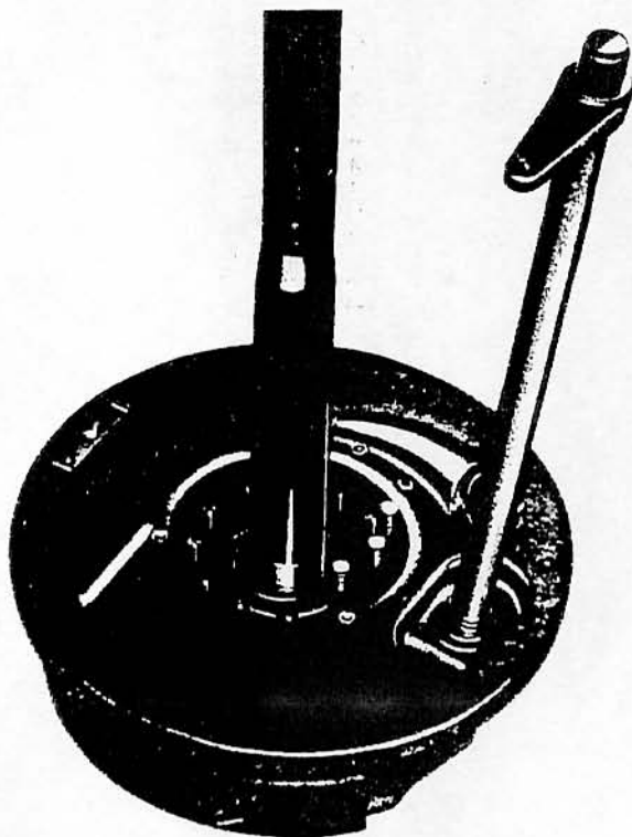
FIGURE 60 REPLACING HALF SHAFT
