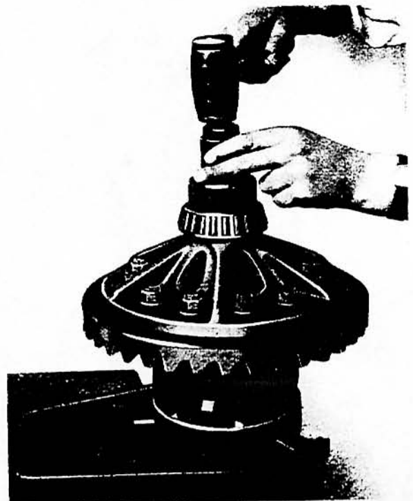
FIG. 28. REPLACING DIFFERENTIAL BEARING CONES
