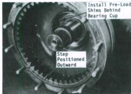
Fig. 232—Planetary ring gear must be positioned with stepped side outward.
