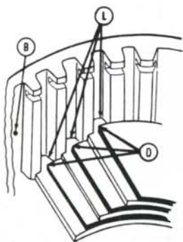
Fig. 208—Cross-sectional view of Multi-Power clutch showing recommended method of assembling clutch discs (D) and clutch plate drive lugs (L) in relation to bleed holes (B) in clutch housing.
