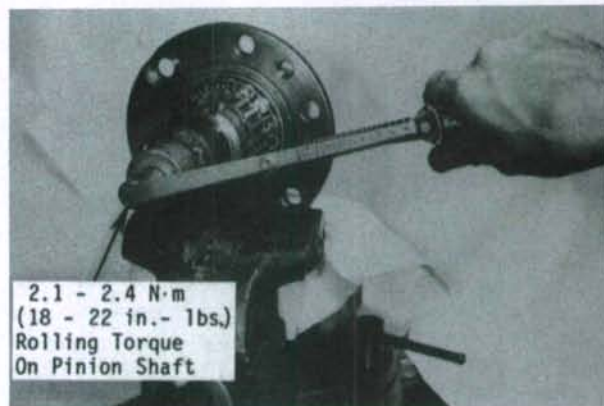
Fig. 225—Use a torque wrench to check pinion shaft rolling torque when adjusting bearing preload.
