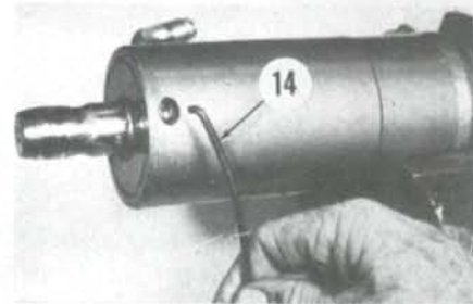
Fig. 19—The hooked end of retaining wire is inserted into hole in bearing cap and cap is turned to pull wire into the groove.
