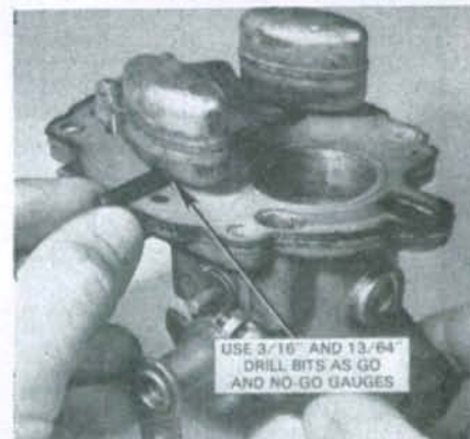
Fig. 118—Float height may be set using 3/16 inch and 13/64 inch drill bits as GO and NO-GO gages.
