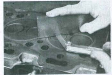
Fig. 89—Valve heads must be recessed the amount specified in text. Measure as shown using straightedge and feeler gage.
