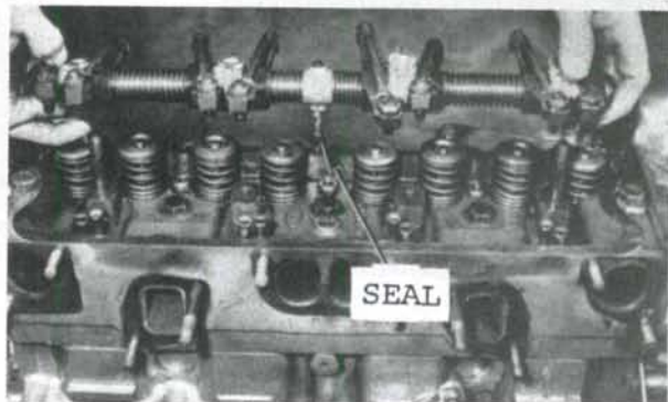
Fig. 26—With TDC timing marks aligned as shown in Fig. 24 and No. 1 piston on exhaust stroke, adjust the indicated valves.
