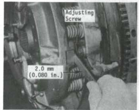
Fig. 173—Adjust pto pressure plate adjusting screws to provide 2.0 mm (0.080 inch) clearance between head of screws and drive plate lugs.
