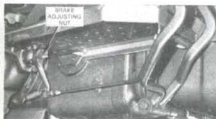
Fig. 235—Turn brake adjusting nut until pedal free play is 70 mm (2-3/4 inches) measured at pedal pad for mechanical brake models.
