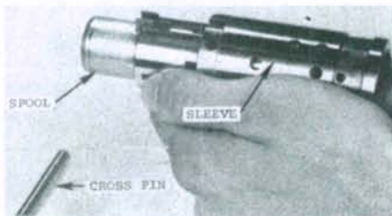
Fig. 11—Spool can be pushed from sleeve after removing cross pin.
