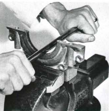
Fig. 42—Use a round bar to bed the asbestos rope seal in retainer half. Refer to text for details.
