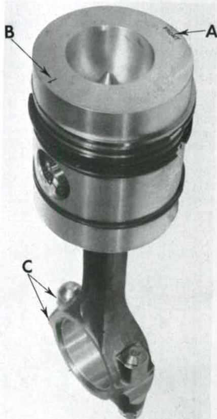
Fig. 99—View of piston and connecting rod correctly assembled with "F" or "FRONT" mark (A), cylinder number (B) and rod correlation numbers (C).
