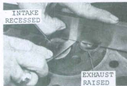
Fig. 22—Intake valve should be recessed 0.91-1.14 mm (0.036-0.045 inch) and exhaust should be raised 1.57-2.06 mm (0.062-0.081 inch) above gasket surface of head.
