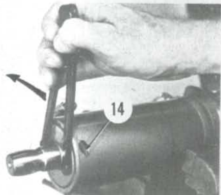
Fig. 20—Turn the bearing cap the direction indicated by arrow to pull retaining wire into groove. Use a screwdriver to start end of wire out of hole and turn end cap opposite direction shown to remove wire.
