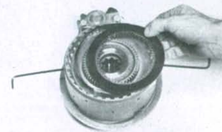
Fig. 252—Insert rods into bleed holes in clutch housing to hold separator springs compressed during clutch assembly. Refer to text.
