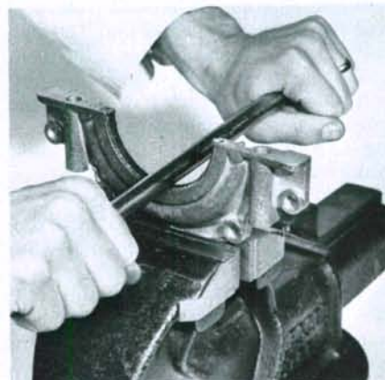
Fig. 105—Use a round bar to seat the asbestos rope seal in each retainer half. Refer to text for details.
