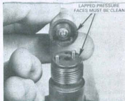
Fig. 131—Be sure lapped surfaces are clean and that locating dowels are perfectly aligned when nozzle body is reinstalled.
