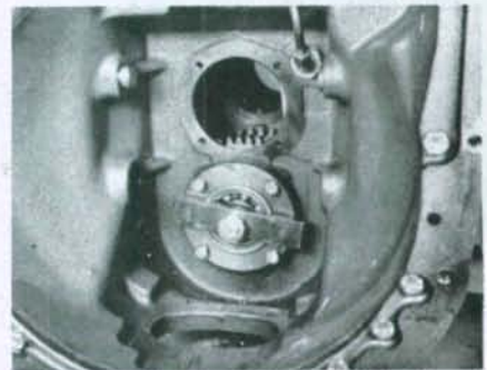
Fig. 192—Pto shaft is drilled and tapped at front end for installation using a suitable puller screw and crossbar as shown.
