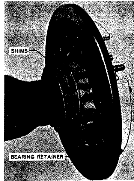
Fig. 319—Axle shaft bearings are adjusted by varying shims located between axle housing and bearing retainer.
