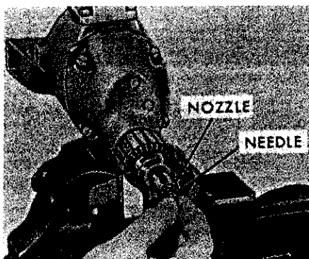
Fig. 133—Chuck small diameter of nozzle in slow speed electric drill to lap needle to nozzle if leak back time is excessive or needle sticks in nozzle. Hold pin end of needle with vise grip pliers.
