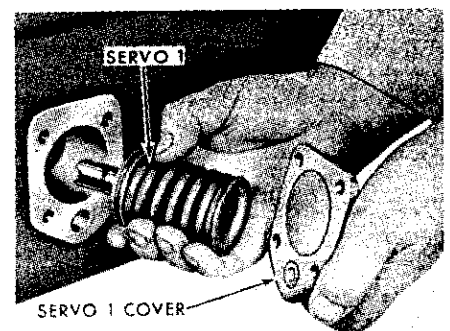
Fig. 258—Removing Servo 1 assembly and cover. Model 5000 is shown for illustrative purposes; however, other models are similar except servo is located at upper side of transmission housing.
