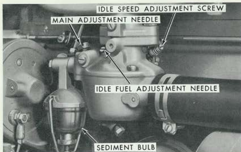
Figure 32 Adjusting the Carburetor (Series 2000)
