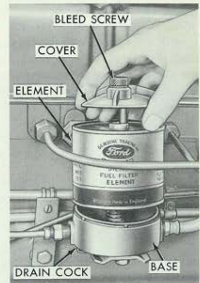
Figure 25 Replacing Diesel Fuel Filter
