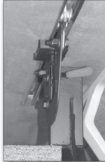
LH & RH Ceiling Clamp Assembly (RH shown)
