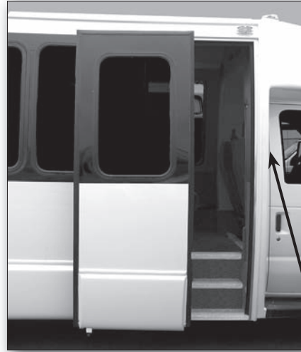
Single Plug Door System (door shown partially open)
