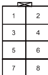
B083 To differential speed switch between wheels
