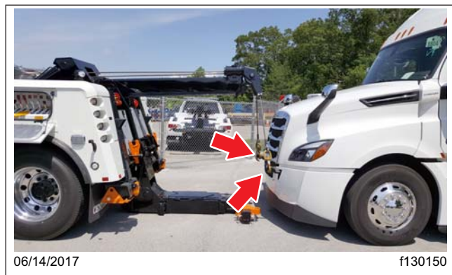
Fig. 24.11, Tow Cables Connected to the Tow Hooks
