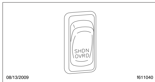
Fig. 10.2, Shutdown Override Switch
