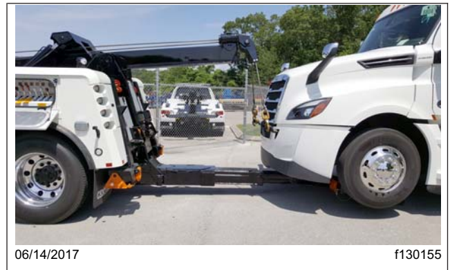
Fig. 24.16, Stinger with Lift Adaptors Under the Axle (tow truck shown)
