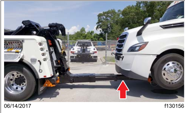
Fig. 24.17, Retracting the Recovery Boom
