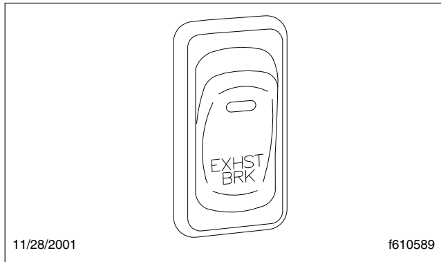
Fig. 5.24, Exhaust Brake Switch
