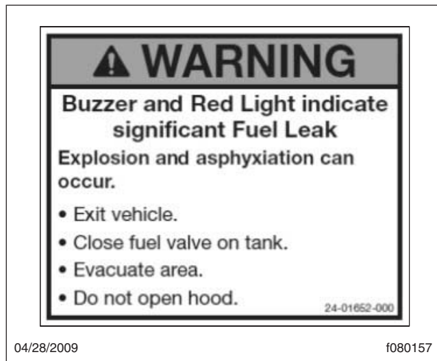
Fig. 19.4, Interior Warning Sticker
