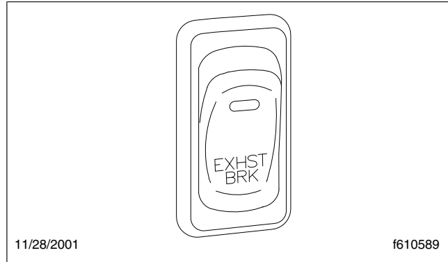
Fig. 10.5, Exhaust Brake Switch
