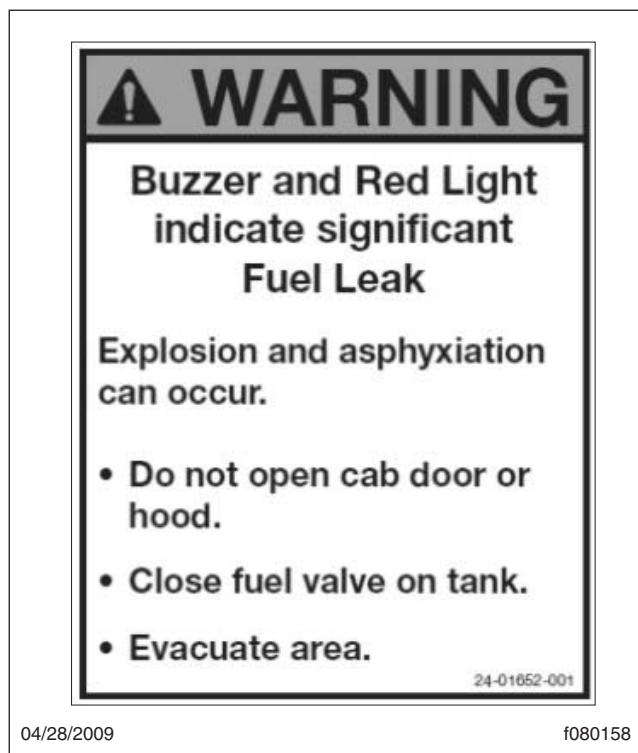
Fig. 19.5, Exterior Warning Sticker
