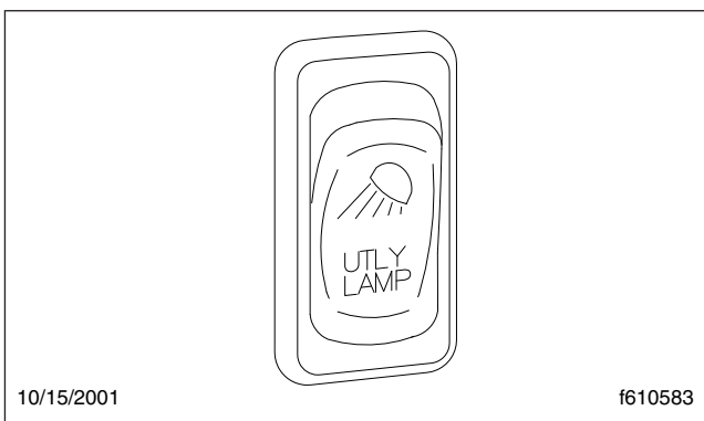
Fig. 5.10, Utility Light Switch
