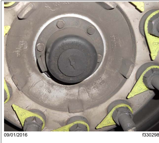
Fig. 10, Normal Oil Venting
