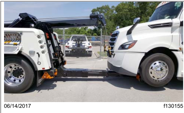
Fig. 21.14, Stinger with Lift Adaptors Under the Axle (tow truck shown)
