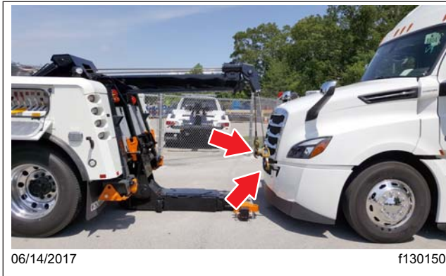
Fig. 21.9, Tow Cables Connected to the Tow Hooks
