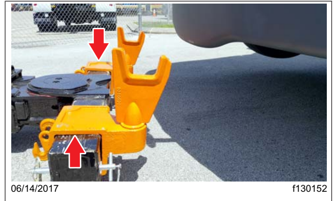
Fig. 21.11, Lift Adaptors Installed on the Crossbar
