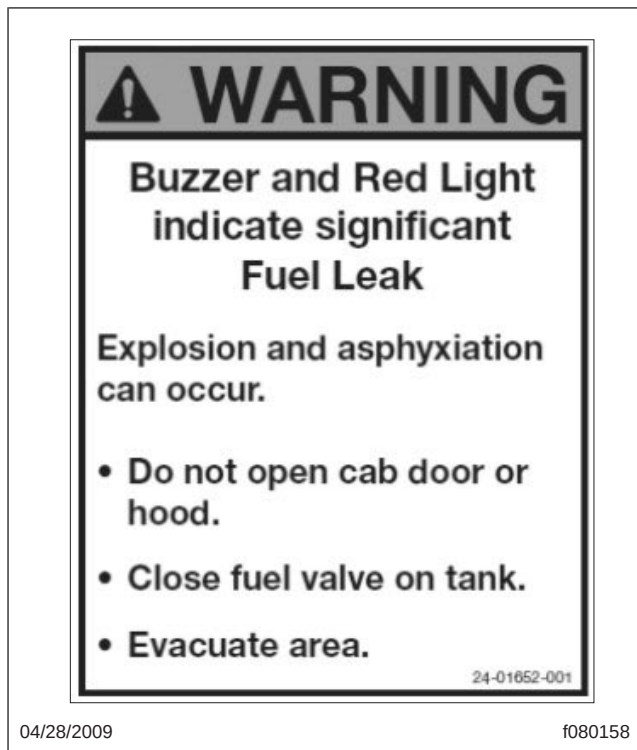
Fig. 16.5, Exterior Warning Sticker
