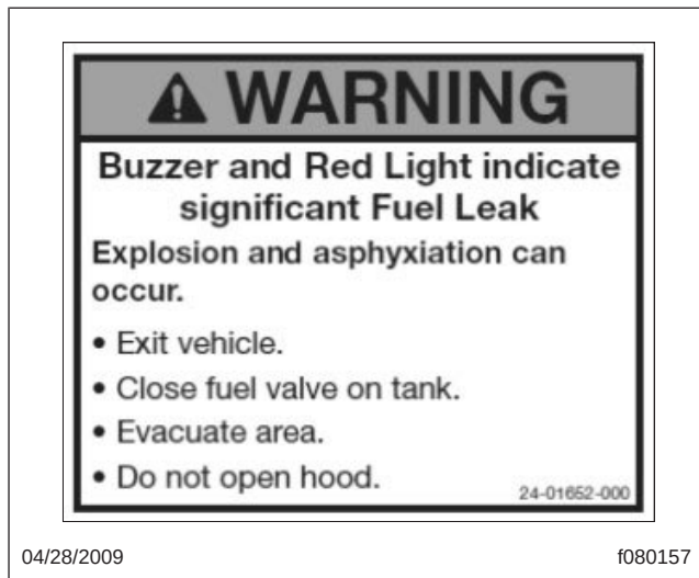
Fig. 16.4, Interior Warning Sticker
