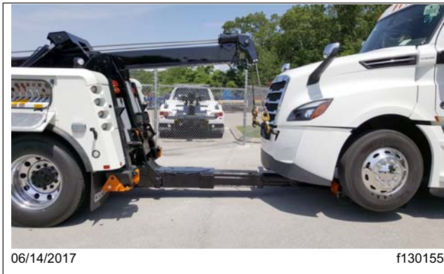
Fig. 13.15, Stinger with Lift Adaptors Under the Axle (tow truck shown)
