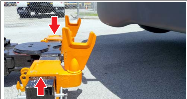
Fig. 13.12, Lift Adaptors Installed on the Crossbar
