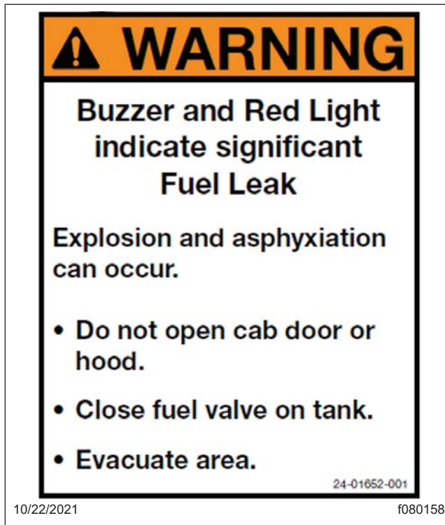
Fig. 16.5, Exterior Warning Sticker
