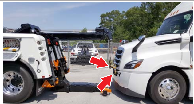
Fig. 13.10, Tow Cables Connected to the Tow Hooks
