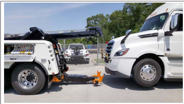
Fig. 13.13, Backing the Tow Truck with Lift Adaptors on the Crossbar
