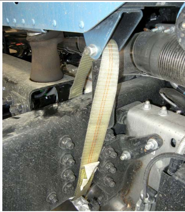
Fig. 23.4, Tension Strap Installed to Hold Down the Cab
