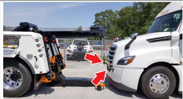
Fig. 24.10, Tow Cables Connected to the Tow Hooks
