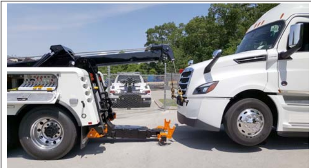
Fig. 24.13, Backing the Tow Truck with Lift Adaptors on the Crossbar
