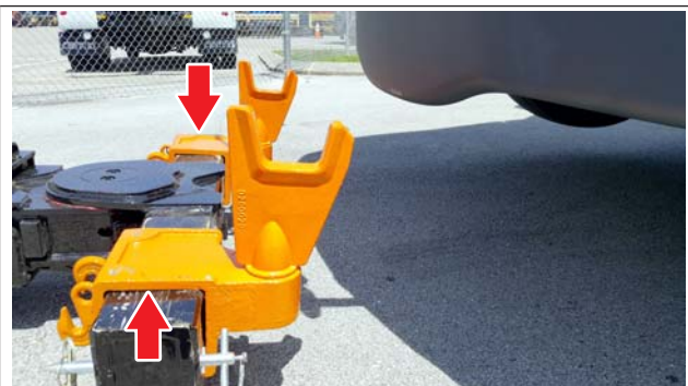
Fig. 24.12, Lift Adaptors Installed on the Crossbar
