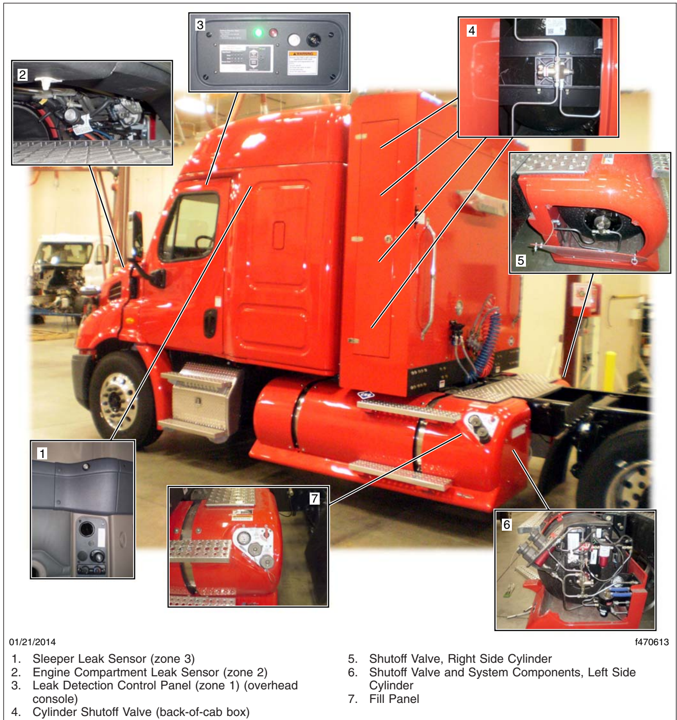
Fig. 25.1, CNG Component Locations
