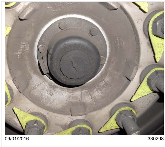
Fig. 9, Normal Oil Venting
