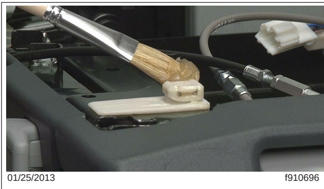
Fig. 7, Applying Grease to Slider Tab
