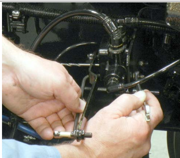
Fig. 2, Holding the height control valve mounting stud in place with an Allen wrench when loosening the nut.
