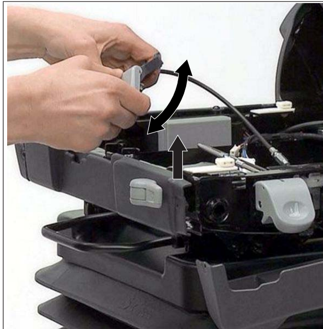
05/01/2014 f910746 Hold the seat tilt lever in the "up" position and pull up the front of the seat frame.
