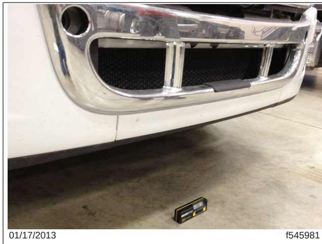
Fig. 1, Measuring the Level on the Surface where the Vehicle is Parked
