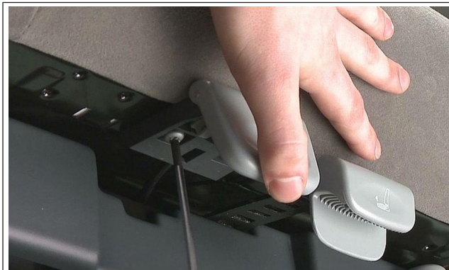
Fig. 2, Removing the Tilt Lever Screws
