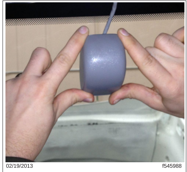
Fig. 2, Removing the Digital Camera
