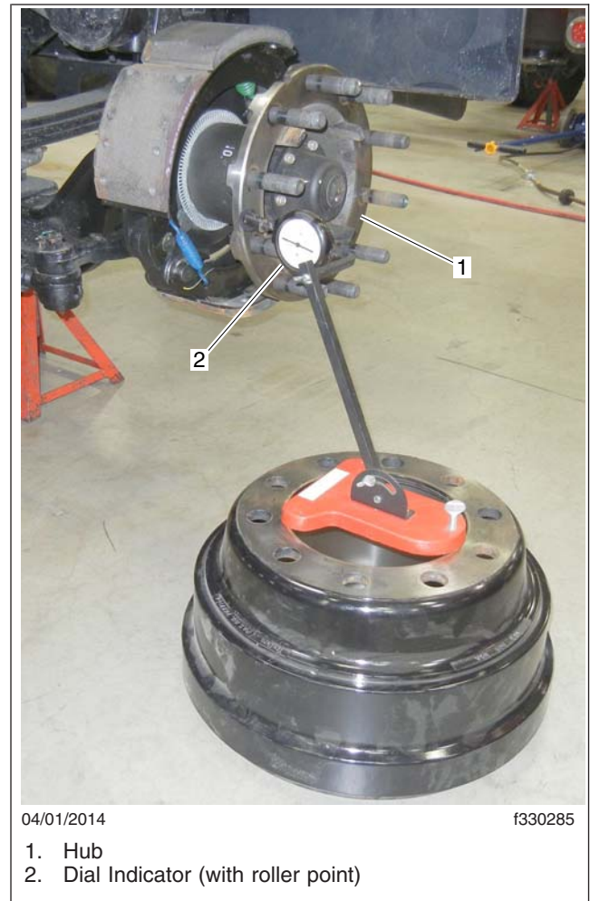
Fig. 1, Setup to Measure Lateral Runout
