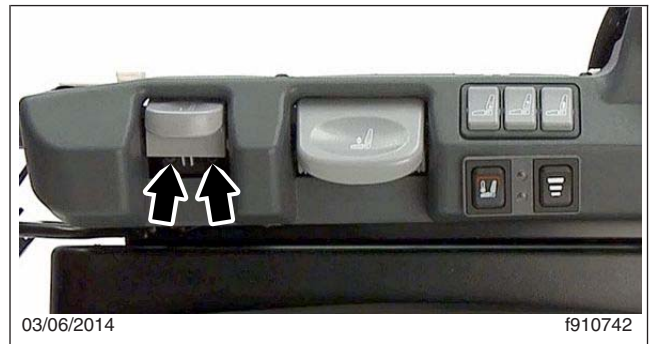
Fig. 10, Shock Absorber Adjustment Lever Mounting Screws
