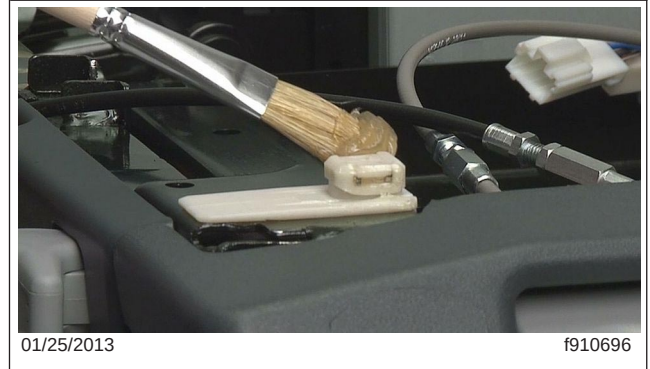
Fig. 3, Applying Grease to Slider Tab
