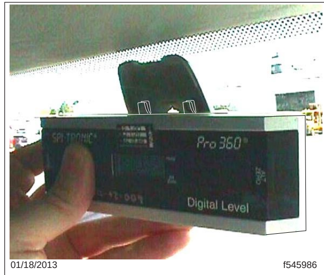
Fig. 6, Checking the Position of the Bracket on the Windshield
