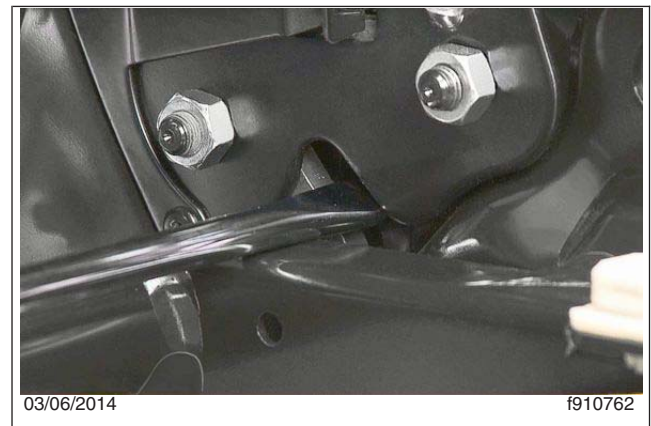
Fig. 3, Jamming the Recline Mechanism
