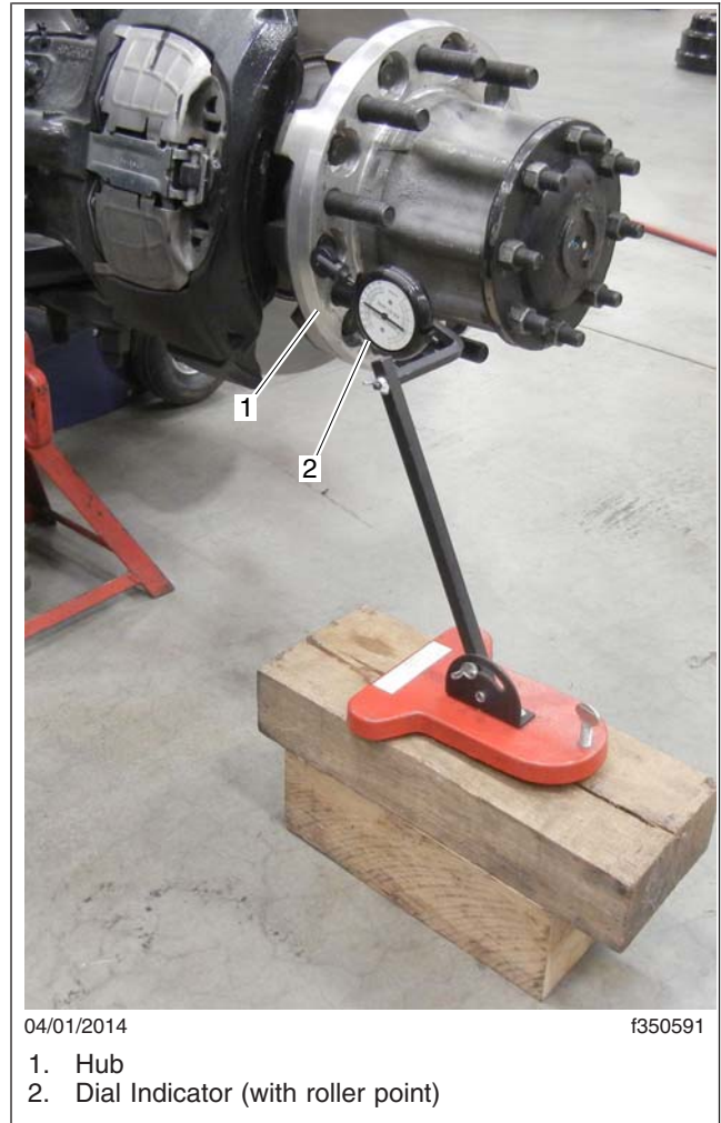
Fig. 1, Setup to Measure Lateral Runout
