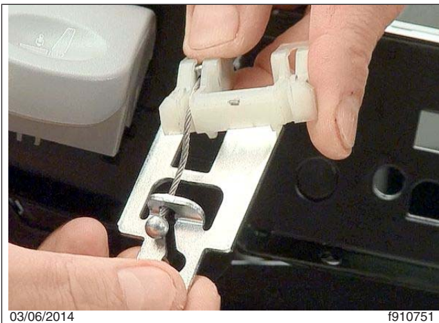
Fig. 19, Hitching the Cable to the Tilt Mechanism
