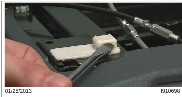
Fig. 2, Removing the Slider Tab Pin
