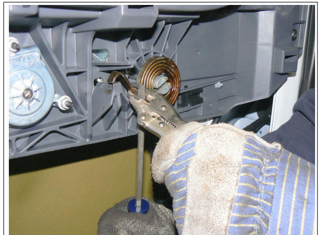
Fig. 2, Unhooking and Unwinding the Counterbalance Spring
