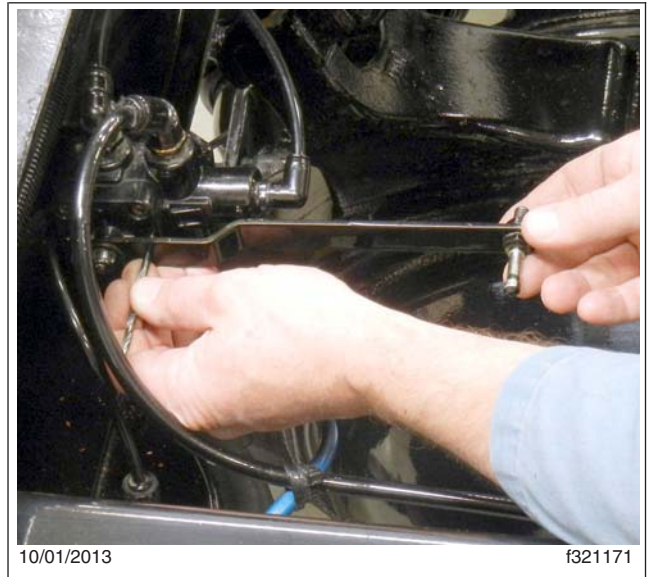
Fig. 1, Inserting a 5/32-inch drill bit or nylon rod to lock the lever in neutral position.
