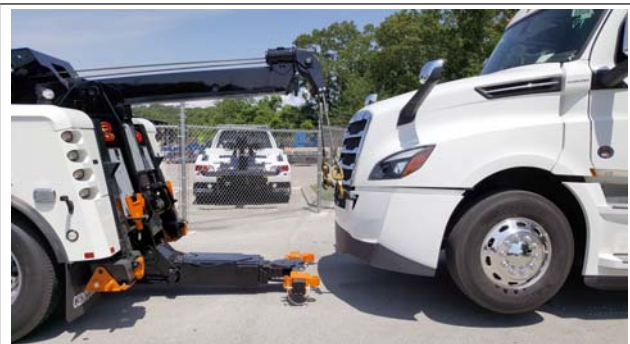
Fig. 13.6, Tow Cables Connected to the Tow Hooks
