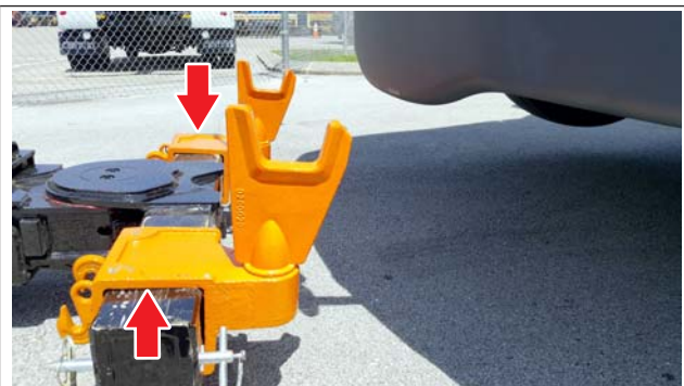
Fig. 13.8, Lift Adaptors Installed on the Crossbar
