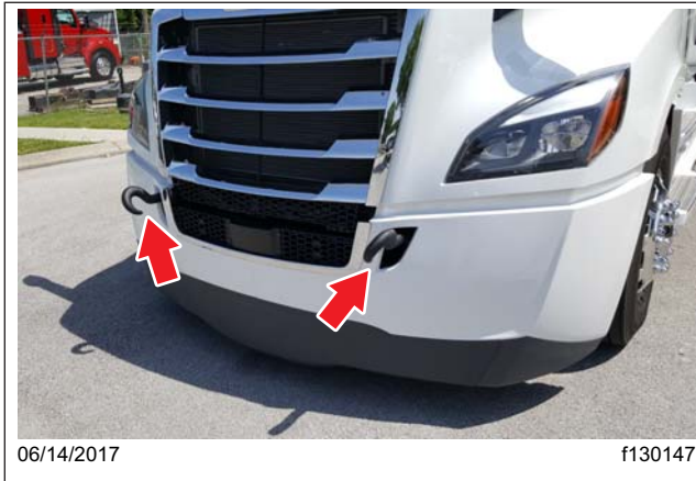
Fig. 13.3, Tow Hooks Installed, Facing Down
