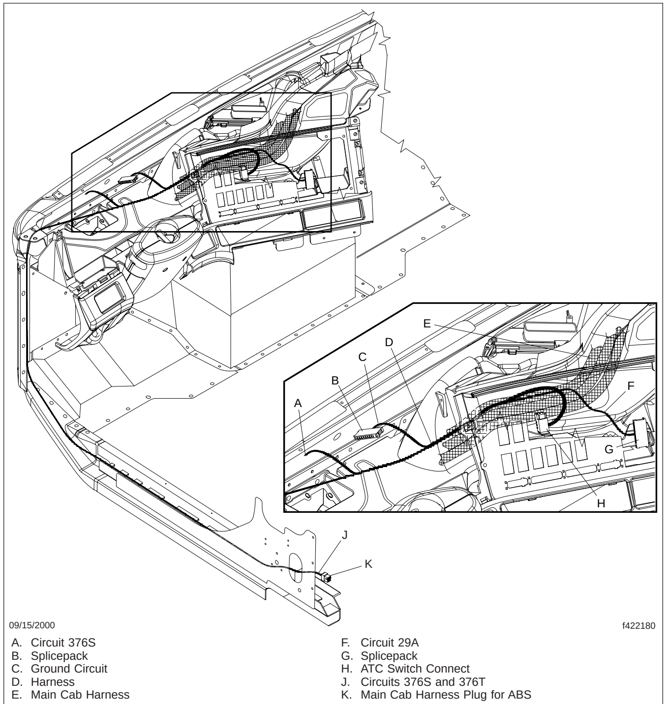
Fig. 10, ATC Switch Harness
