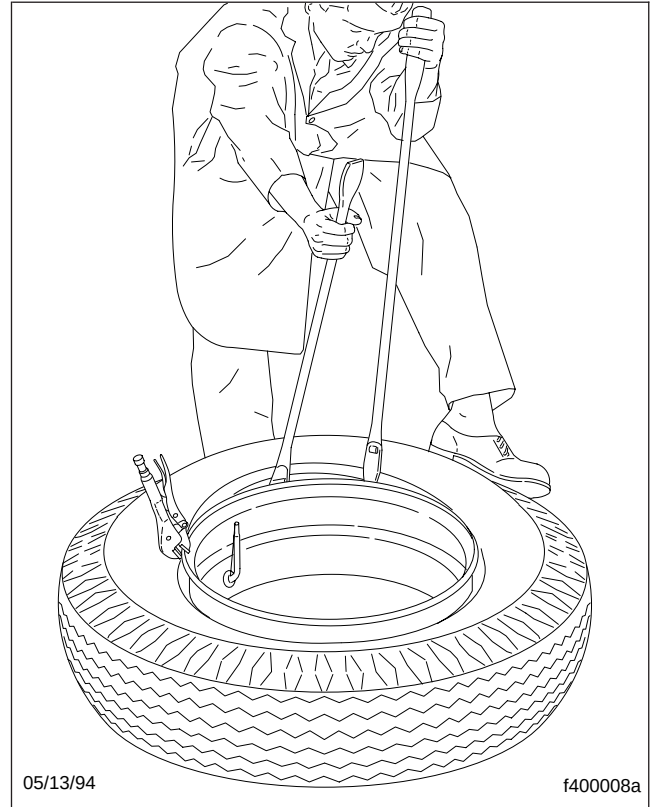
Fig. 6, Working the Upper Bead into the Rim
