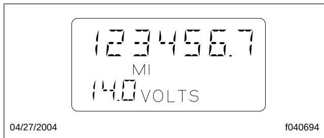
Fig. 3, Message Display Screen with Integrated Digital Voltmeter
