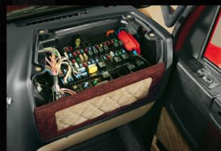
Power Distribution Module (PDM)
