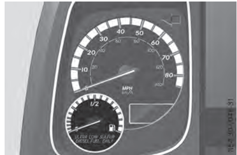
Fuel gauge (example: instrument cluster with large screen)
