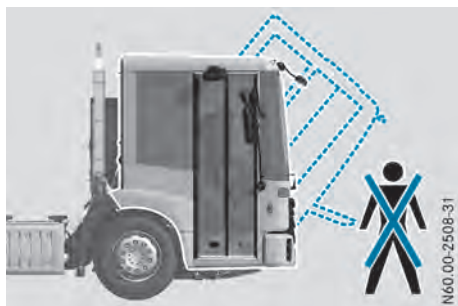
Tilting area of the cab
