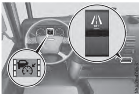
Lane Keeping Assist button and display
