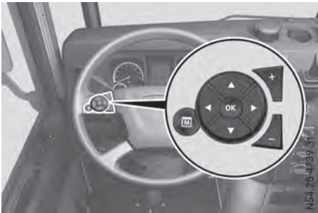
Left button group on the multifunction steering wheel
