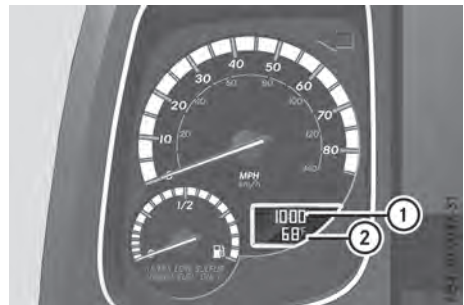
Clock and outside temperature (example: instrument cluster with large screen)
