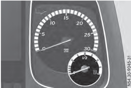
DEF display (example: instrument cluster with large screen)
