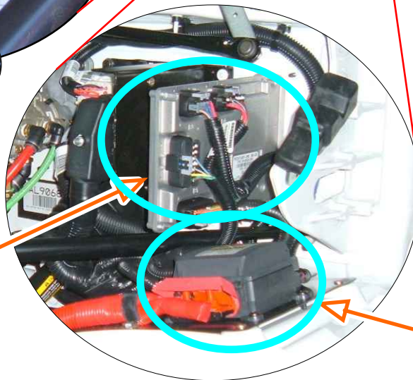
Power Distribution (Module 285 PDM)
