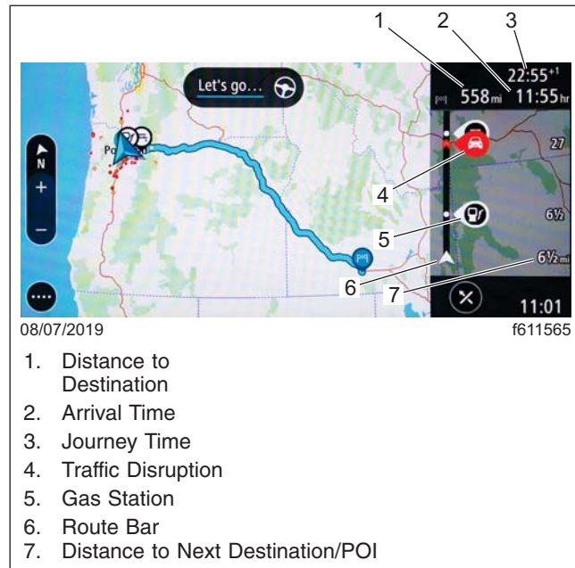
Fig. 7.22, Example of a Wide Route Bar - ICC5
