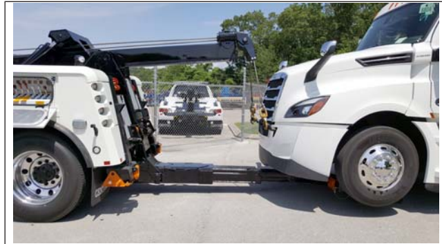
Fig. 26.12, Stinger with Lift Adaptors Under the Axle (tow truck shown)
