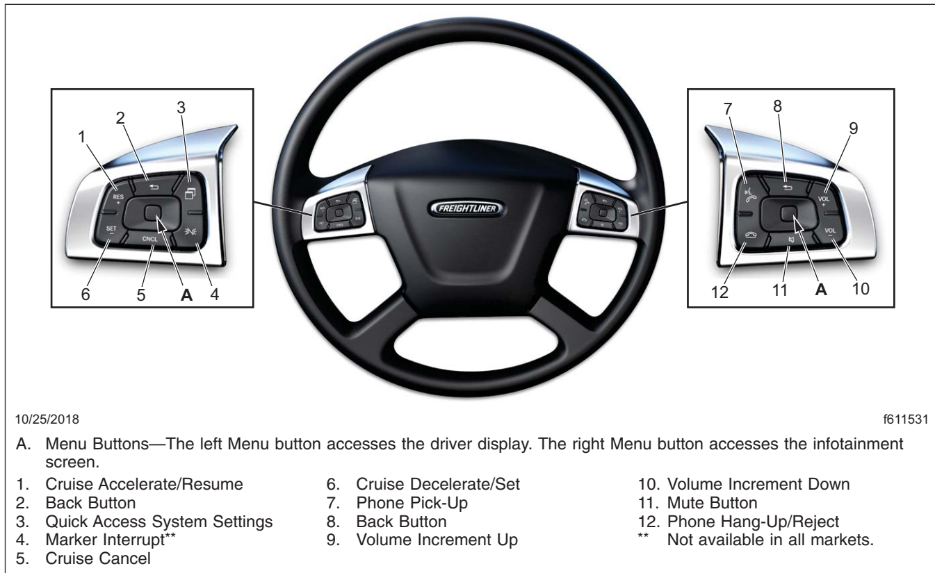
Fig. 3.52, Steering-Wheel-Mounted Optical Finger Navigation Control (OFN) buttons - ICC5
