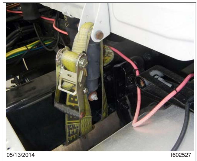
Fig. 26.16, Tension Strap Installed to Hold Down the Cab
