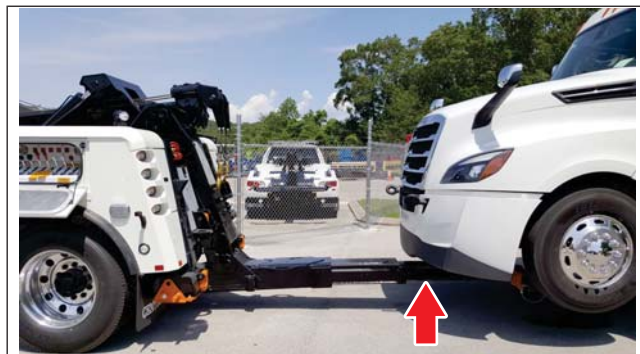
Fig. 26.13, Retracting the Recovery Boom
