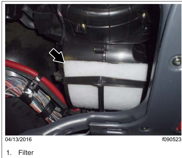
Fig. 4, Cab Recirculation Air Filter
