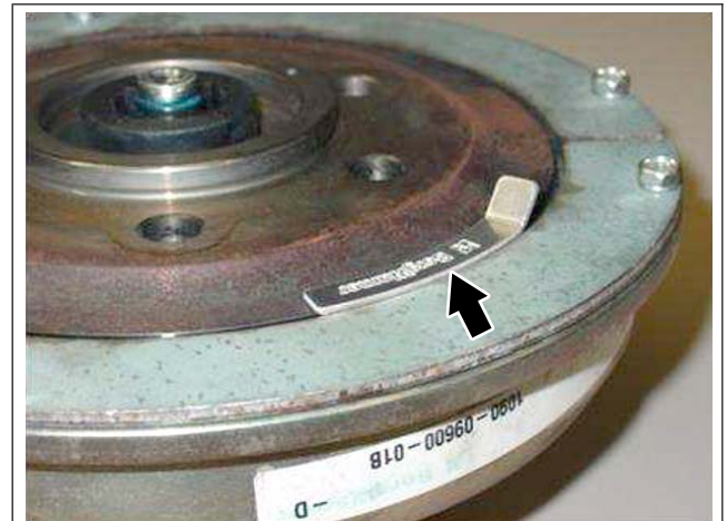
Fig. 4, Tool Below Retainer Plate, Liner Life Remaining
