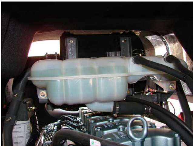
Under Mounted Expansion Tank
