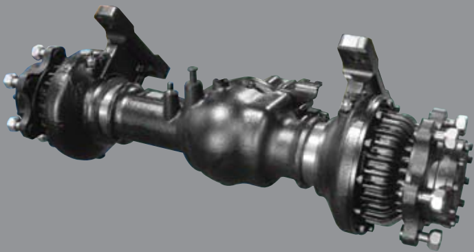
Highly Durable Split Type Drive Axle The bevel gear set and hub reduction axle smoothly delivers desired torque to the drive wheels with wet disc drive.
