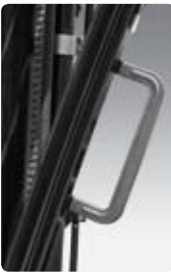
Large Footboard & Hand Grip Wide "open" step offers convenience and safety when entering and exiting truck. Step is high grade durable plastic entrance step of additional safety when entering and exiting forklift.
