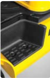
Large Footboard & Hand Grip Wide "open" step offers convenience and safety when entering and exiting truck. Step is high grade durable plastic entrance step of additional safety when entering and exiting forklift.
