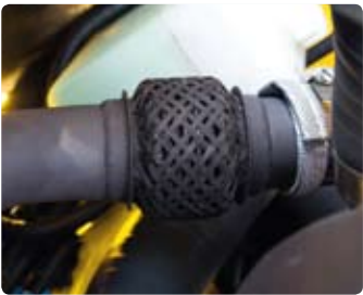
Expansion Bellows The expansion bellows absorbs vibration and reduces noise generated from the exhaust gas system and also extends the life cycle of exhaust gas system.
