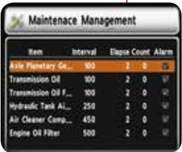
Maintenance Management Display
