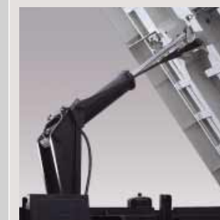
Marrel-type (HD270) dump mechanism
