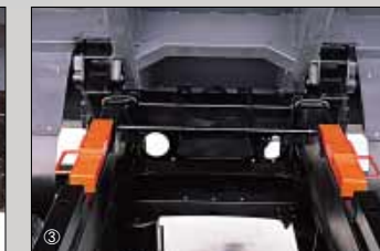
Marrel-type (HD270) dump mechanism
