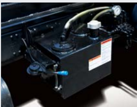
Oil Tank & Control Lever
