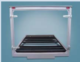
Rear door frame thickness (2.3mm → 3.2mm)
