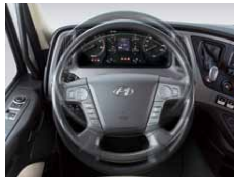
Steering wheel (Including pneumatic tilt and telescopic function)
