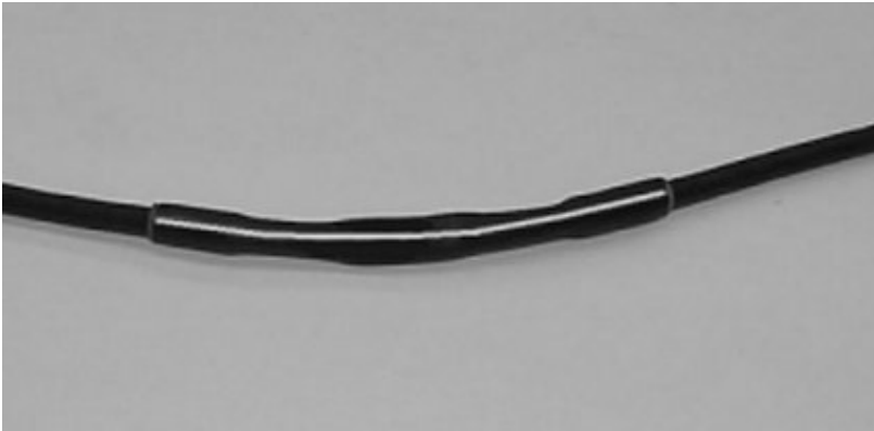
Figure 11 Center Heat Shrink Tube Over Cable
