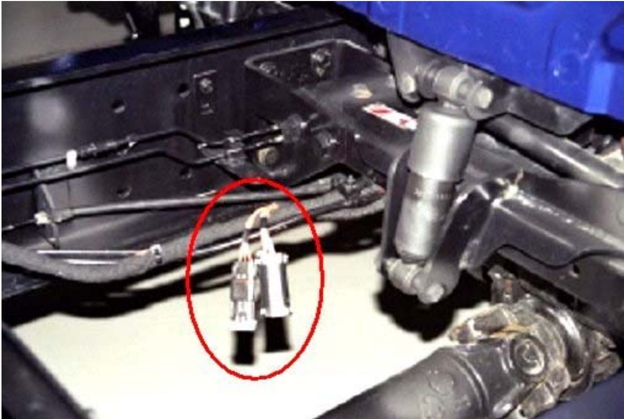
Figure 64 7-Way and 3-Way Connectors for 08HAB (Back of Cab)
