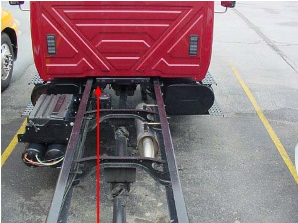
Figure 80 Arrow Indicates Location of Work Light Connector (Straight Truck)
