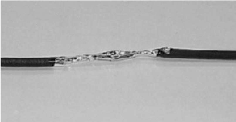
Figure 10 Center Heat Shrink Tube Over Cable
