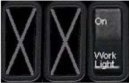
Figure 79 Work Light Switch in 3-Switchpack Below and Left of Gauge Cluster
