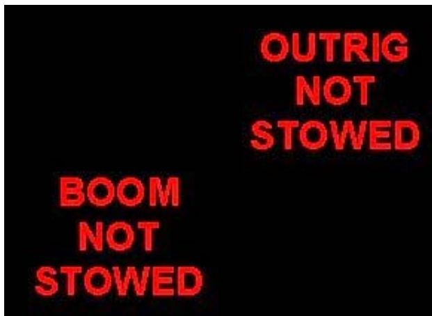
Figure 137 Gauge Cluster Display of “Outrig Not Stowed” and “Boom Not Stowed”
