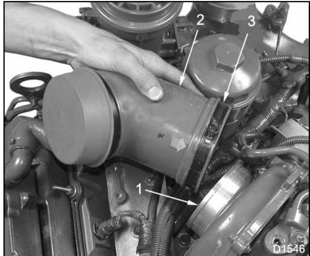
Figure 50 Air inlet duct
