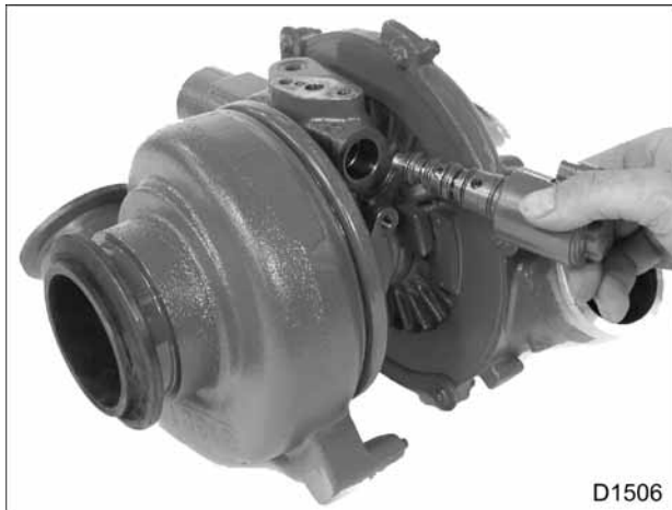
Figure 48 VGT control valve
