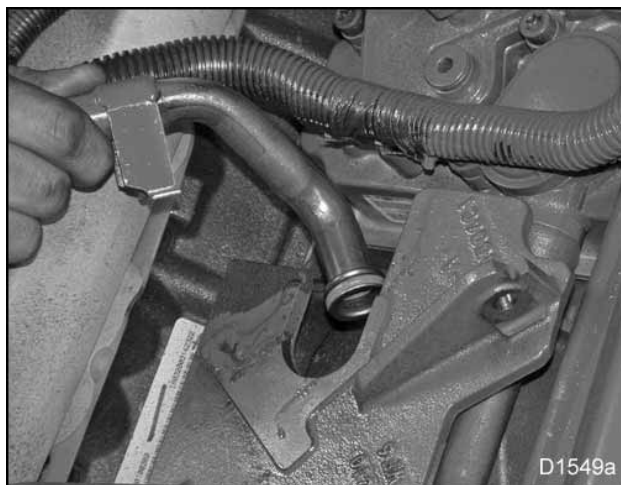
Figure 59 Removal of oil drain tube for VGT
