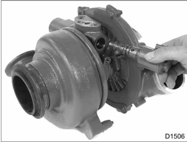
Figure 48 VGT control valve
