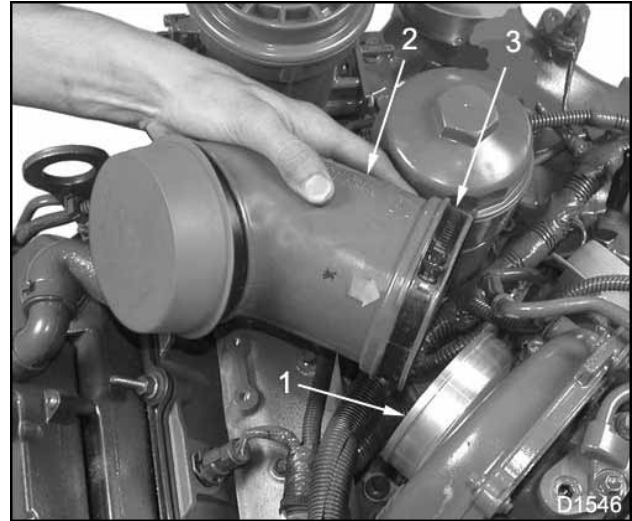
Figure 50 Air inlet duct
