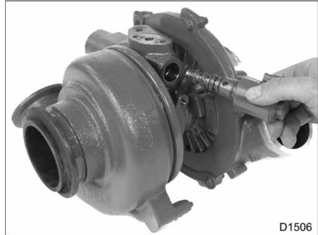
Figure 77 VGT control valve
