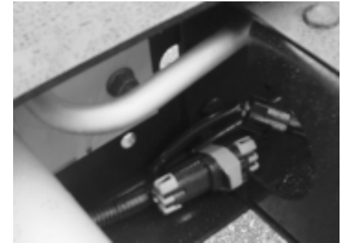
Back Buzzer circuit connector located on LH rail aft of last cross member
