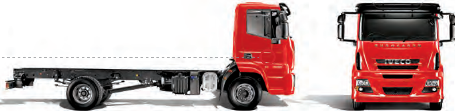
CAB WITH 2 ACCESS STEPS for 12- to 18-tonne versions
