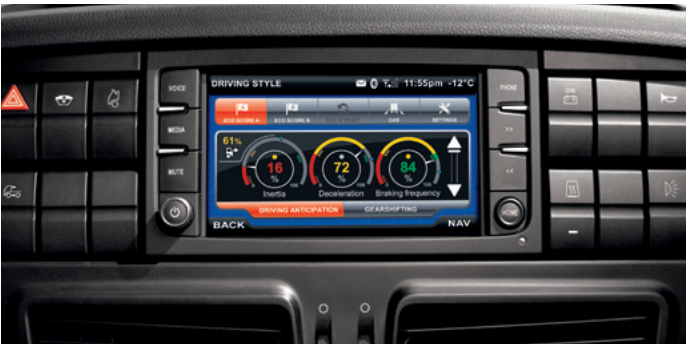
EACH OF THESE INDEXES IS DISPLAYED TO THE USER IN REAL TIME WITH AN ANALOGUE INDICATOR SHOWING THE PERCENTAGE IN THE CENTRE. THE HIGHER THE MARK, THE BETTER THE DRIVING IN TERMS OF FUEL SAVING.
