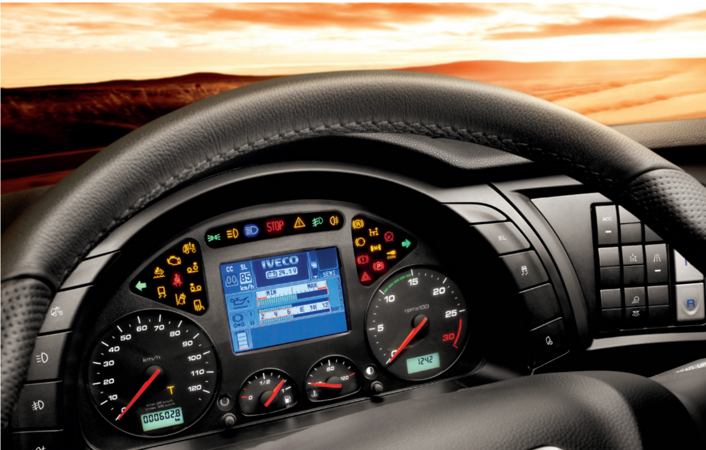
ECOSWITCH LIMITS THE TOP SPEED AND OPTIMISES DRIVELINE PERFORMANCE ON THE BASIS OF THE VEHICLE'S ACTUAL LOAD.
