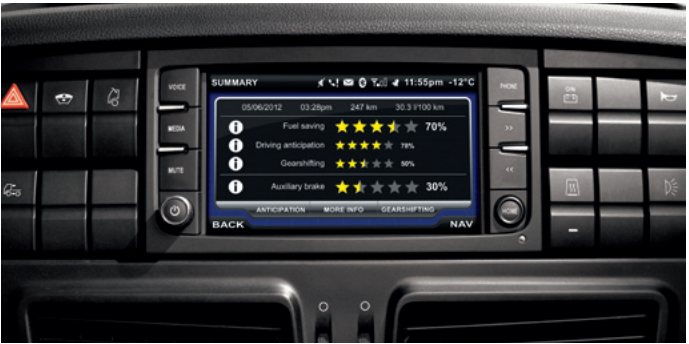
AT THE END OF EACH TRIP, THE DRIVER CAN VIEW A SUMMARY OF ALL THE PERFORMANCE INDEXES ON THE MONITOR, EXPRESSED IN PERCENTAGES AND DISPLAYED IN GRAPH FORM.
