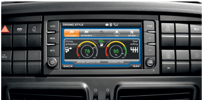
DRIVING STYLE EVALUATION: THE SYSTEM PROCESSES THE DATA ACQUIRED FROM THE ENGINE, VEHICLE AND GPS USING AN ADVANCED ALGORITHM (DEVELOPED BY IVECO) THAT EVALUATES THE DRIVER'S FUEL SAVING PERFORMANCE. THE EVALUATION IS BASED ON A SET OF INDEXES IN A THREE-LEVEL TREE STRUCTURE, TAKING INTO ACCOUNT THE DIFFICULTY OF THE MISSION.
