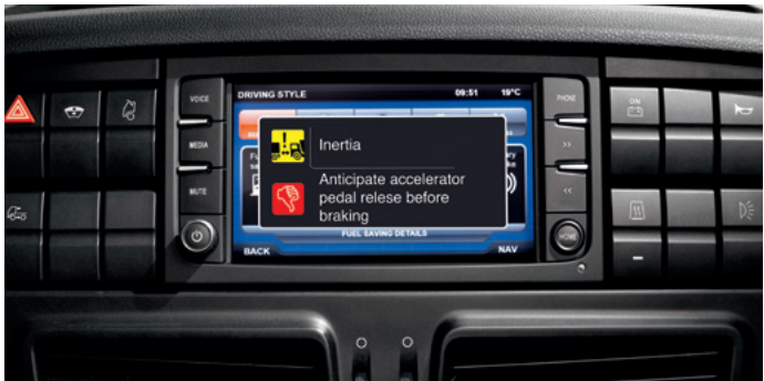
ALSO WHILE THE VEHICLE IS RUNNING, FUEL-SAVING SUGGESTIONS APPEAR ON THE IVECONNECT SCREEN (USE OF GEARS, BRAKING, ENGINE BRAKING, ACCELERATION AND INERTIA).
