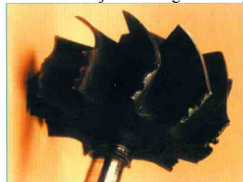
Turbine impeller damaged by particles
