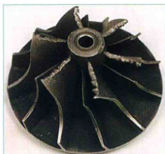
Compressor impeller damaged by particles
