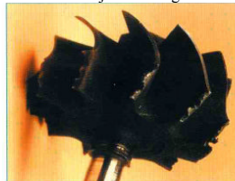
Turbine impeller damaged by particles
