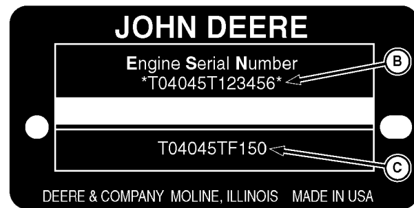
Dubuque Engine Serial Number Plate
