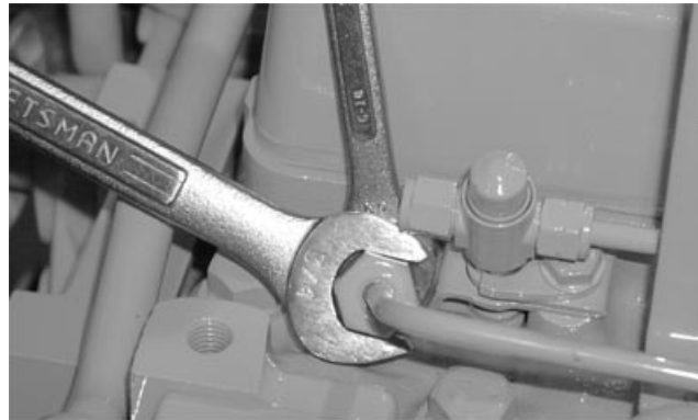
Nozzle Fuel Pressure Line
